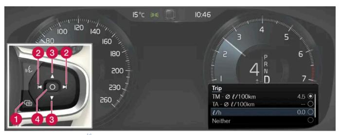
Open and navigate in the app menu [1] using the right-hand steering wheel keypad.
