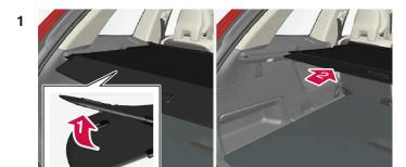
In the fully open position, push the cover's handle slightly upward with e.g. your elbow.
