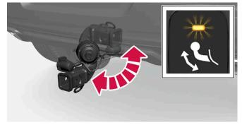
Secure the hitch into position by pushing it back to its retracted position under the bumper, where it will lock into place.
