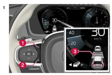
Controls for setting a time interval.
