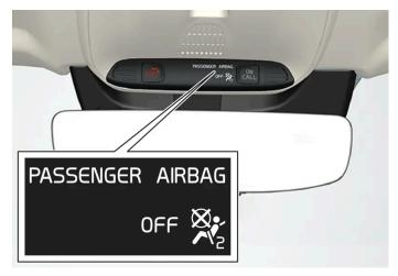
Occupant Weight Sensor (OWS) indicator light
