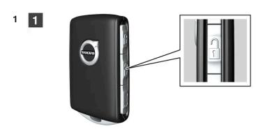
1 Unlock the vehicle using the key. Charging will stop.
