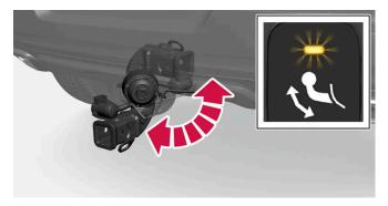
➤ The hitch will fold out and down to an unlocked position – the indicator lamp will flash orange. The hitch is ready to be moved to the locked position.
