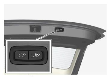
Location of button(s) on underside of tailgate.
