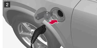
Open the charger door and remove the charging socket's protective cover. Push the charging handle all the way into the vehicle's socket.
