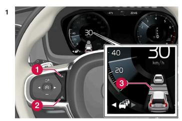
Controls for setting a time interval.
