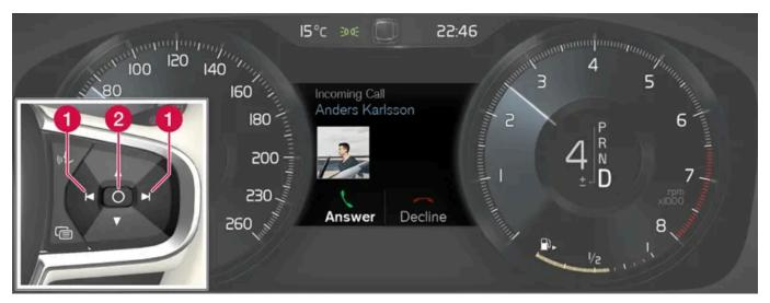
Examples of messages in the instrument panel and the right-side steering wheel keypad. The illustration is generic - details may vary according to vehicle model.
