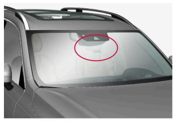
Location of front camera and radar sensor
