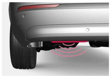
The sensor is located to the left of center under the rear bumper<sup>[1]</sup>.
