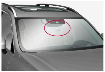
Location of front camera and radar sensor
