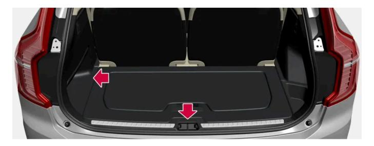
The cargo compartment capacity can be considerably increased by folding down the backrests in the second and third rows\* of seats. To make loading and unloading easier, the rear section of the vehicle can be raised and lowered using the level control function\*. Use the load anchoring eyelets or grocery bag holders to help secure objects in place, and the retractable cargo compartment cover\* to help conceal objects in the cargo compartment.
