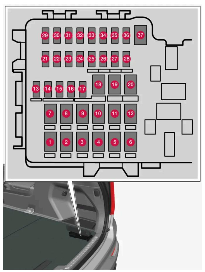
The fuse box is located under the storage compartment on the right-hand side.
