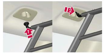
Press one of the grid's hooks into the larger hole in the ceiling bracket (1).
