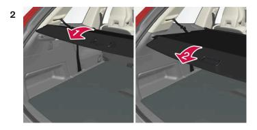
Grasp the handle and pull the cover out and above the side panels in the cargo compartment. Pull the cover to its end position.
