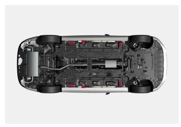
The vehicle has outer lifting points for smaller lifts, and inner lifting points for larger lifts with a garage hoist, lifting arms, etc.
