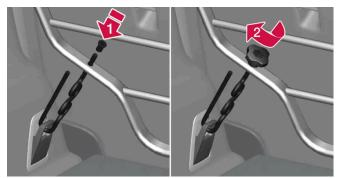
Attach the mounting bracket's hook through the cargo anchoring eyelet near the floor of the cargo compartment and insert the threaded section of the bracket through the grid's lower attachment hole (1).
