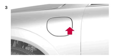
Press the rear edge of the charger door to open the charging socket and remove the charging socket's protective cover [2].
