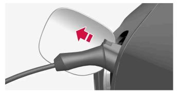
Press the release button on the charging cable's handle. The handle will be released/unlocked. Remove the cable from the vehicle's charging socket, put the socket's cover back in place and close the charger door.
