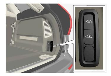
Use the buttons in the cargo compartment to raise or lower the rear section of the vehicle to facilitate loading or unloading the vehicle or connecting or disconnecting a trailer.
