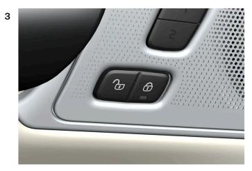
Press the central locking button, as shown in the illustration.
