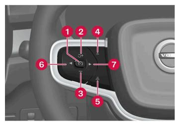
Buttons for speed-controlling functions
