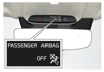
Occupant Weight Sensor (OWS) indicator light
