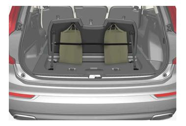
There are two grocery bag holders and an elastic band [2] in the hatch in the cargo compartment floor. The strap can be attached in four different positions.
