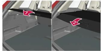
Grasp the handle and pull the cover out and above the side panels in the cargo compartment. Pull the cover to its end
