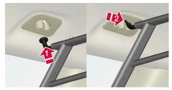
Press one of the grid's hooks into the larger hole in the ceiling attachment point (1).
