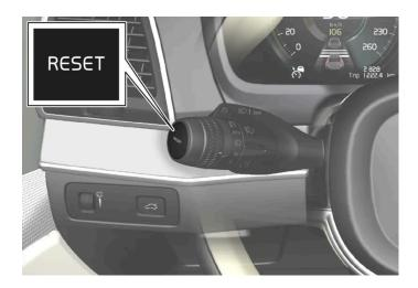
1 Reset all information in trip odometer TM (i.e. mileage, average fuel consumption, average speed and driving time) by pressing and holding the RESET button on the left-hand steering wheel lever.
