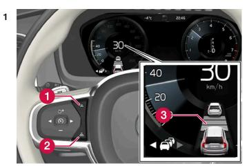
Controls for setting a time interval.
