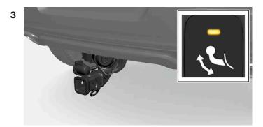
Move the hitch to its end position, where it will lock in place – the indicator lamp will glow steadily orange.
