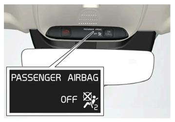
Occupant Weight Sensor (OWS) indicator light
