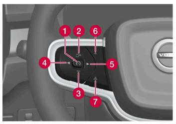
Buttons for speed-controlling functions
