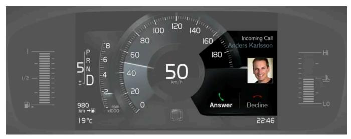
Example of message in an 8-inch instrument panel. The illustration is generic - details may vary according to vehicle model.
