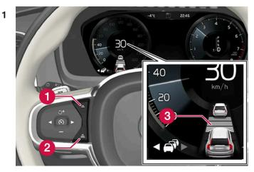
Controls for setting a time interval.
