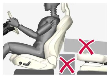
Do not place any objects on the floor behind or under the front seats or on the rear seat that could prevent WHIPS from functioning correctly.
