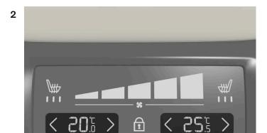
Temperature controls on the rear climate panel of the tunnel console.
