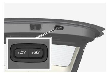
Location of button(s) on underside of tailgate.
