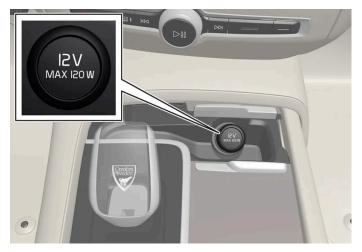
Front electrical outlet in the tunnel console for vehicles with wireless phone charger  ${}^\star$  .
