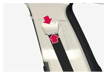
Press the button on the seat belt holder and move the belt up or down.
