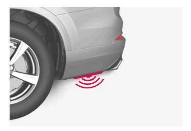
To activate opening and closing using a foot movement on a vehicle with skid plate, make a kicking motion from the side of the vehicle. One of the vehicle's remote keys must be within range (approx. 1 meter (3 feet)) for opening and closing to be possible.
