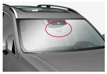
Location of front camera and radar sensor
