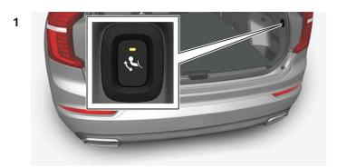
Open the tailgate. There is a button for operating the hitch on the right-hand side at the rear of the cargo compartment. Steady orange illumination from the indicator light in the button shows that the folding function is active.
