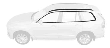
Components that should be washed with a cleaning product with a pH value between 3.5 and 11.5.
