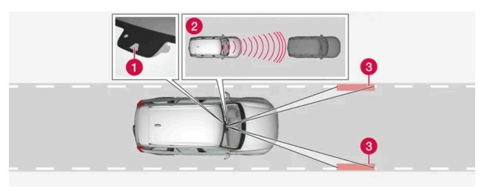
The camera/radar sensor monitors the distance to the vehicle ahead and detects lane markings.
