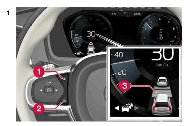
Controls for setting a time interval.
