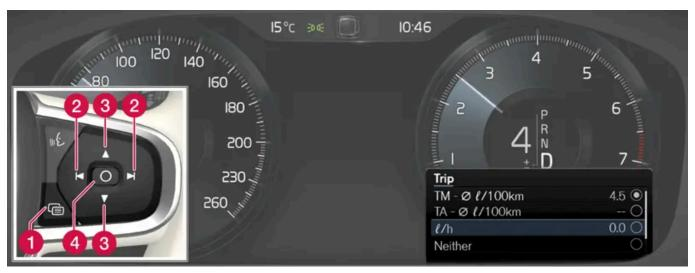
Open and navigate in the app menu [1] using the right-hand steering wheel keypad.
