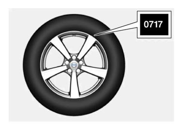
Tires are perishable goods. After a few years, they will begin to harden and their friction properties will gradually deteriorate. Always replace tires with the freshest tires possible. This is particularly important for snow tires. A series of numbers is imprinted on the sidewall of the tire. The last four digits in the series is the Department of Transportation (DOT) stamp and indi-
