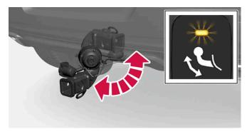
> The hitch will fold out and down to an unlocked position – the indicator lamp will flash orange. The hitch is ready to be moved to the locked position.
