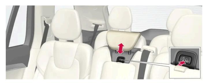
To lower the restraint, press and hold the button (located between the backrest and the head restraint, see illustration) while carefully lowering the head restraint.
