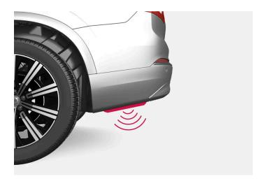
To activate opening and closing using a foot movement on a vehicle with skid plate, make a kicking motion from the side of the vehicle. One of the vehicle's keys must be in range, about 1 meter (3 feet), for activation to be possible.
