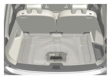
If the vehicle is a mild hybrid, it instead has a 48 V support battery located under the cargo compartment. The battery and the box over it may only be handled by authorized workshop personnel.
