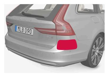
Keep the marked area clean (on both the left and right sides of the vehicle) $^{[2]}$ .
