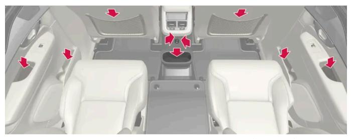
Storage compartment in the door panel, cup holders at the bottom of the tunnel console, storage pocket\* in the front seat's backrest and USB ports in the tunnel console.
