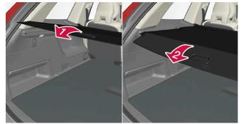
Grasp the handle and pull the cover out and above the side panels in the cargo compartment. Pull the cover to its end position.
