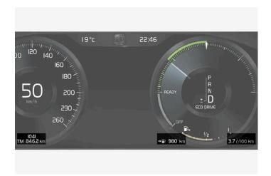
Example of trip computer information in a 12-inch instrument panel\*. The illustration is generic - details may vary according to vehicle model.
