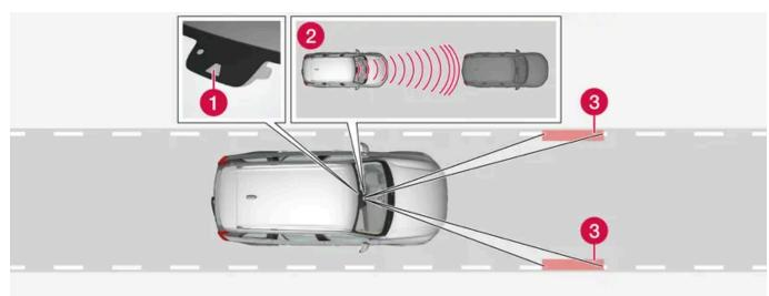
The camera/radar sensor monitors the distance to the vehicle ahead and detects lane markings.
