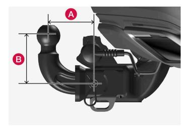
The ball mount must fall within the geometric limits for the towbar, for both distance (A) and height (B). Geometric limits are described on a type plate located on the towbar.
