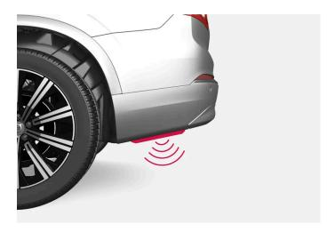
To activate opening and closing using a foot movement on a vehicle with skid plate, make a kicking motion from the side of the vehicle. One of the vehicle's keys must be in range, about 1 meter (3 feet), for activation to be possible.
