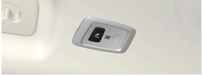
In vehicles with panoramic roofs\*, there are two lamp units, one on each side of the ceiling. [2]
