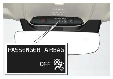
Occupant Weight Sensor (OWS) indicator light
