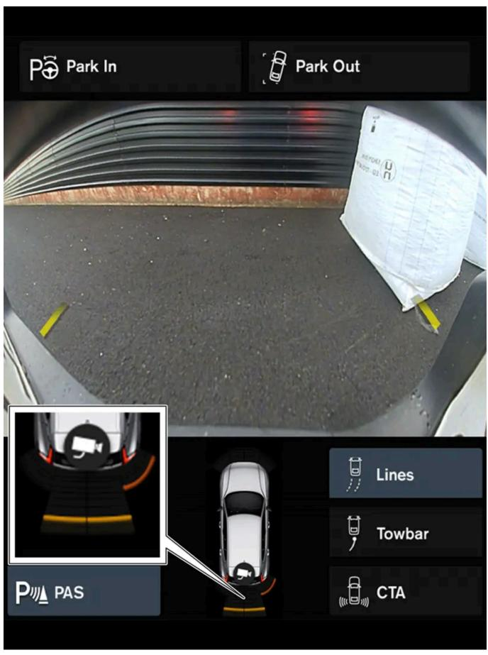
The screen can display colored sensor fields on the vehicle symbol.
