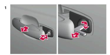
Pull the front left-hand door handle to its end position to access the lock cylinder.
