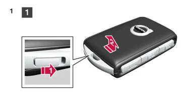
Hold the key with the front side (with the Volvo logo) facing up and move the button on the key ring bracket to the right. Slide the front cover slightly upward.
