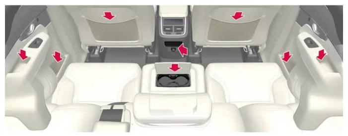
Storage compartment in the door panel, cup holders\* in the center seat's backrest, storage pocket\* in the front seat's backrest and USB ports in
