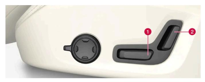
1 Move the passenger seat forward/rearward by moving the control forward/rearward.
