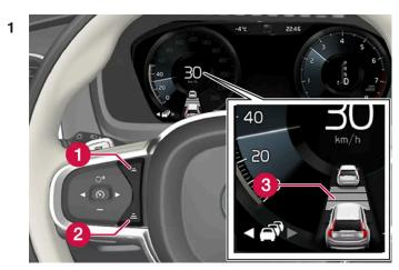
Controls for setting a time interval.
