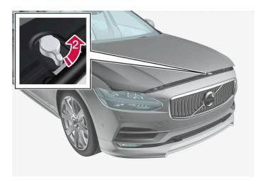
Turn the handle under the front edge of the hood counterclockwise to release the catch and lift the hood.
