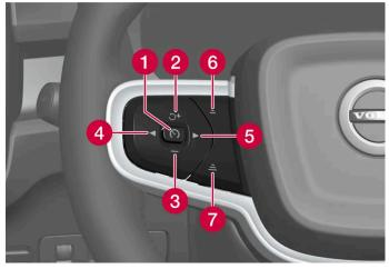
Buttons for speed-controlling functions
