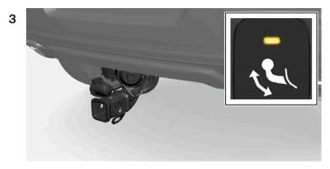
Move the hitch to its end position, where it will lock in place – the indicator lamp will glow steadily orange.
