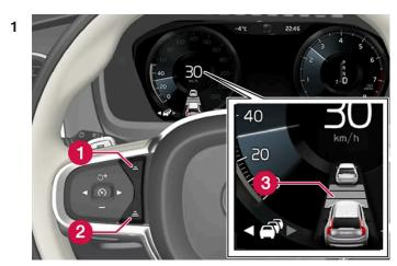
Controls for setting a time interval.
