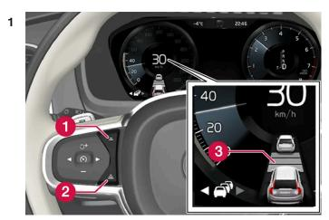
Controls for setting a time interval.
