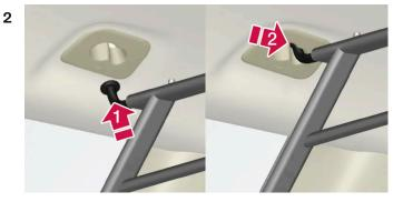
Press one of the grid's hooks into the larger hole in the ceiling bracket (1). Grasp the grid near the hook and pull/push it into the smaller hole (2).
