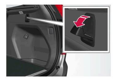
There are two fold-out holders in the side panels, one on each side of the cargo compartment.
