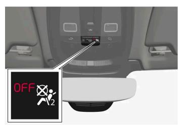
Occupant Weight Sensor (OWS) indicator light
