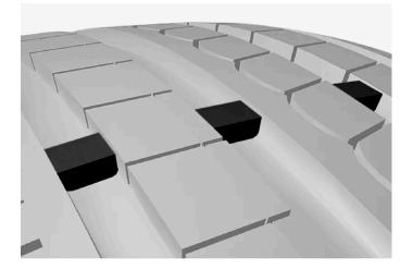
The tread wear indicator is a narrow elevated strip running across the tire's longitudinal tread grooves. The letters TWI (Tread Wear Indicator) are visible on the side of the tire. When approximately 1.6 mm (1/16 inch) is left on the tread, the tread will be at the same height as the tread wear indicator. Replace the tire as soon as possible. Tires with low tread offer very poor traction in rain or snow.
