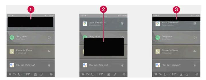
**1** Shown at the top of the center display. Requires immediate action and may have up to three buttons allowing the user to manage the message. Dismiss by swiping right or left. The message will then be saved in Notifications view.
