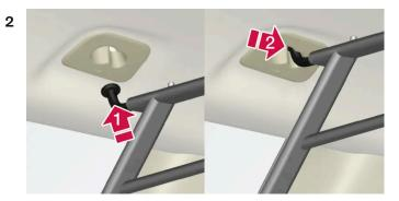
Press one of the grid's hooks into the larger hole in the ceiling bracket (1).
