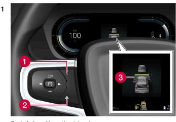
Controls for setting a time interval.
