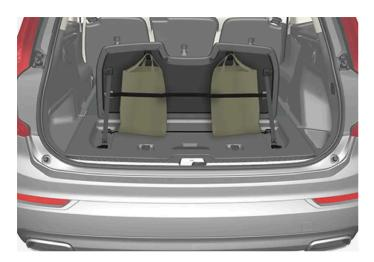
There are two grocery bag holders and an elastic band<sup>[2]</sup> in the hatch in the cargo compartment floor. The strap can be attached in four different positions.
