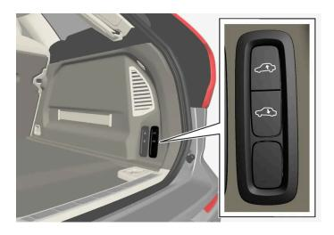
Use the buttons in the cargo compartment to raise or lower the rear section of the vehicle to facilitate loading or unloading the vehicle or connecting or disconnecting a trailer.
