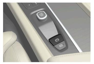
The parking brake controls are located in the tunnel console between the seats.
