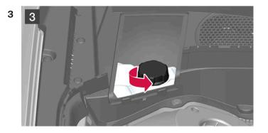
Unscrew the expansion tank cap and fill coolant as needed. The level should be between the MIN and MAX marks on the expansion tank.
