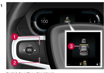
Controls for setting a time interval.
