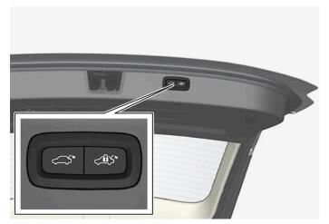
Location of button(s) on underside of tailgate.
