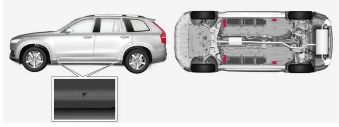
Arrows along the lower edges of the sides of the vehicle indicate the location of the jack attachment points/lifting points (shown in red).
