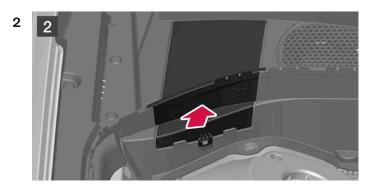
Remove the plastic cover by folding out the catch and lifting the cover upward.
