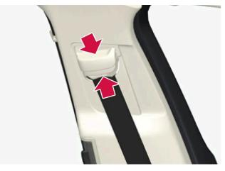
Press the button on the seat belt holder and move the belt up or down.
