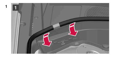
Lift the rubber strip by pressing it inward into the engine compartment.
