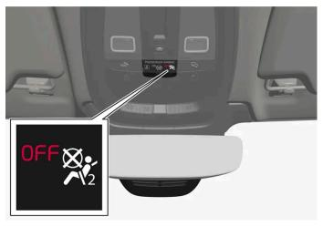
Occupant Weight Sensor (OWS) indicator light
