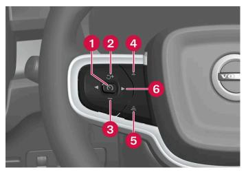
Buttons for speed-controlling functions
