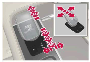
Gear selector and gear selector positions overview.
