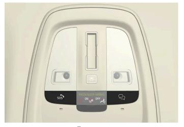
The functions are available via  $\Re$  and the SOS buttons in the overhead console.
