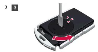
Turn the battery cover counterclockwise to the OPEN position. Use a screwdriver, coin or similar.
