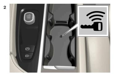
Place the key on the key symbol in the backup reader in the tunnel console's cup holder.
