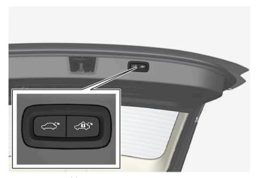
Location of button(s) on underside of tailgate.
