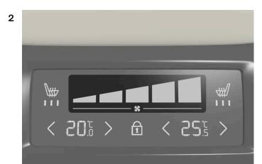
Blower controls on the rear climate panel of the tunnel console.
