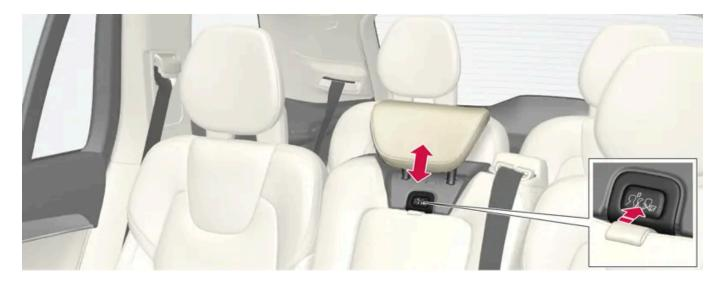
To lower the restraint, press and hold the button (located between the backrest and the head restraint, see illustration) while carefully lowering the head restraint.
