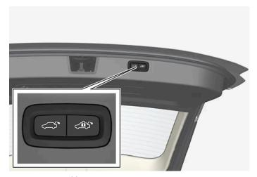
Location of button(s) on underside of tailgate.
