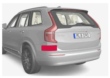
Keep the marked area clean (on both the left and right sides of the vehicle).
