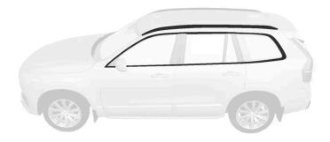
Components that should be washed with a cleaning product with a pH value between 3.5 and 11.5.
