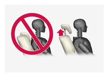
The center head restraint should be adjusted to suit the passenger's height. The entire back of the head should be covered if possible. Manually move the restraint up or down as needed.
