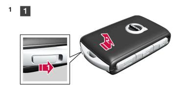
Move the catch next to the key ring bracket to the side and slide the front cover away from the bracket.
