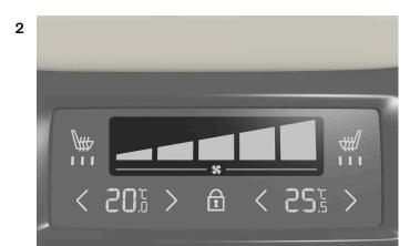
Blower controls on the rear climate panel of the tunnel console.
