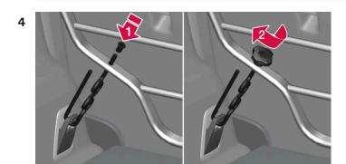
Attach the mounting bracket's hook through the cargo anchoring eyelet near the floor of the cargo compartment and insert the threaded section of the bracket through the grid's lower attachment hole (1).
