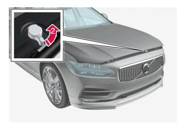
Turn the handle under the hood counterclockwise to release the catch and lift the hood.
