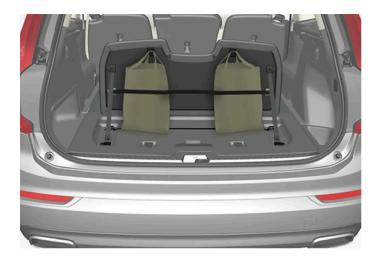
There are two grocery bag holders and an elastic band [2] in the hatch in the cargo compartment floor. The strap can be attached in four different positions.
