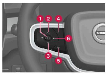
Buttons for speed-controlling functions
