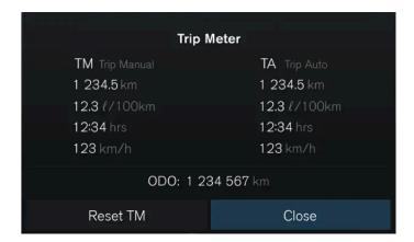
Your vehicle has a trip meter and an odometer. The trip meter can show information on the vehicle's driving distance and time, as well as your average fuel consumption and driving speed.
