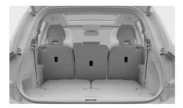
The top tether attachment point locations for the outer second-row seats are indicated by the top tether symbol.
