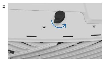
Locate the second lever below the front edge of the hood and rotate it counter-clockwise.
