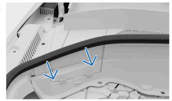
The coolant container is located in the upper-left corner of the engine compartment, underneath a panel hatch. Pull the rubber seal toward the engine compartment to access the hatch.
