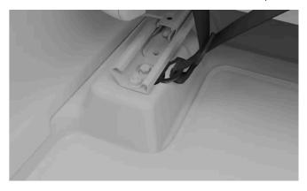
Tighten the straps to make the safety net tight and more secure.
