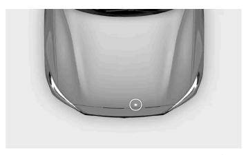
The second lever is below the front edge of the hood, on the driver's side.
