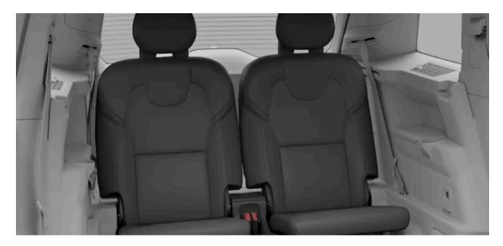
The backrests and headrests can fold in one motion to give you more stowing space. The headrest folds down automatically when the backrest is lowered.
