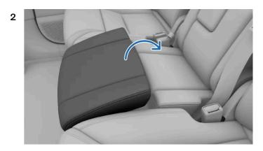
Using one hand on the front of the child seat and one on the rear, guide the child seat upwards and back all the way to the backrest of the seat.
