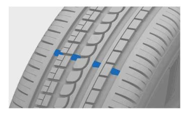
The narrow grooves that run lengthwise across the tire's tread pattern are tread wear indicators. On the side of the tire are the letters TWI [1].
