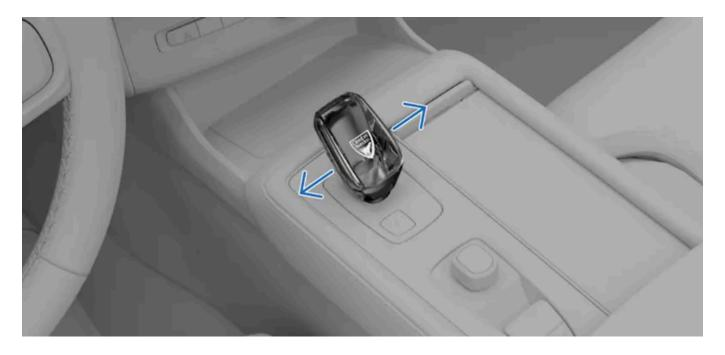
After selecting gear M, you can manually shift gears by moving the gear selector to the left or right.
