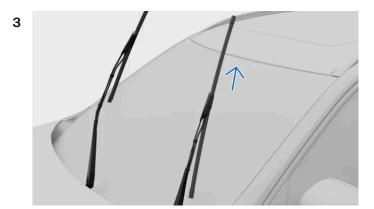
Press the button on the wiper arm and remove the wiper blade by pulling it upward.
