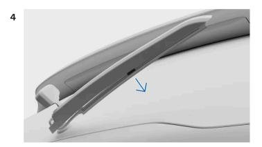
Pull the blade down until it loosens and comes away from the wiper arm.
