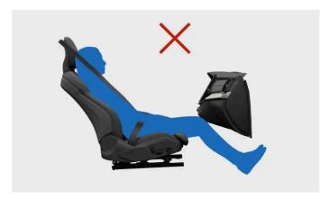
Do not tilt the backrest to a lying position. The seat belt must remain tensioned against the shoulder.
