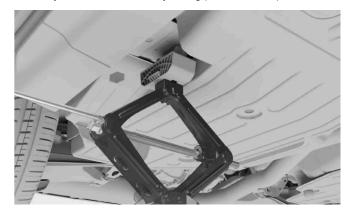
**9** Raise the vehicle to an appropriate height. Do not raise it higher than necessary for the work you're doing.
