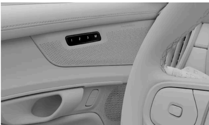
Location of the preset seat adjustment buttons
