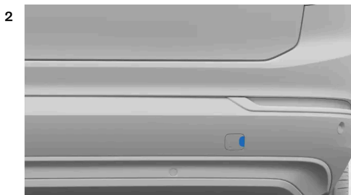
Rear towing eye fastening cover
