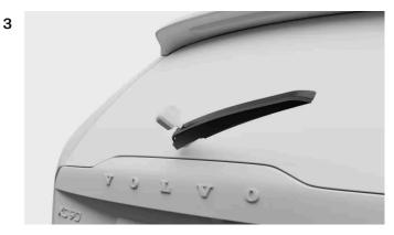
Grasp the center of the wiper arm and lift it up and away from the rear windshield. You may feel some resistance halfway – this is the lock position. You need to pull the wiper arm past the lock position so that it doesn't fall back onto the windshield
