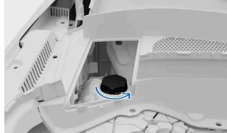
Unscrew the coolant reservoir cap.
