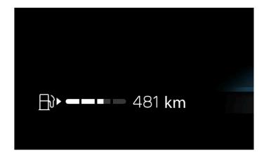
Your range is primarily related to the amount of fuel left in the tank and your driving practices, but external conditions can also be a factor. The fuel meter and expected range are displayed in the instrument panel.
