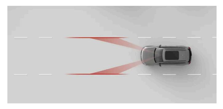
When lane keeping aid is enabled, the vehicle can alert you if you are about to drift out of your lane, and it can ask you to steer the vehicle with attention. It can also perform steering interventions. The lane keeping aid relies on the vehicle's forward-facing camera to identify road markings and your position in the lane.
