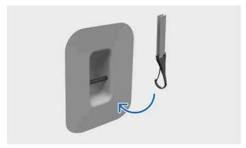
Fastening tether to top tether attachment point
