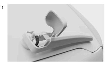
Find the plastic cover where the wiper arm attaches to the vehicle. Loosen the side of the cover closest to you first and then the side furthest away from you. Lift the plastic cover all the way. This will give you access to the hose connector.
