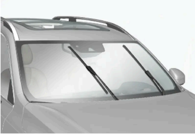
Viskerblade i servicestilling.
