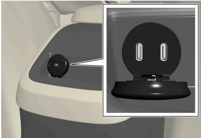
USB-poorten (type C) in tunnelconsole, achterbank.
