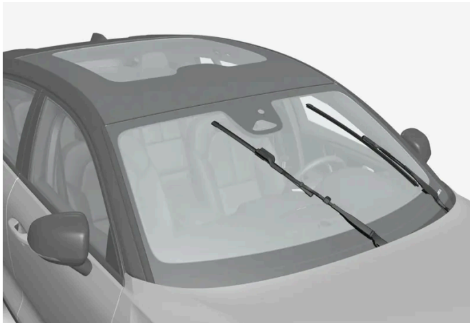
Viskerblader i servicestilling.
