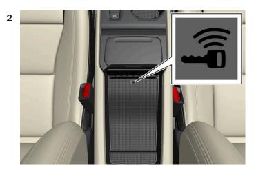
Place the key on the key symbol in the backup reader in the tunnel console's storage compartment.
