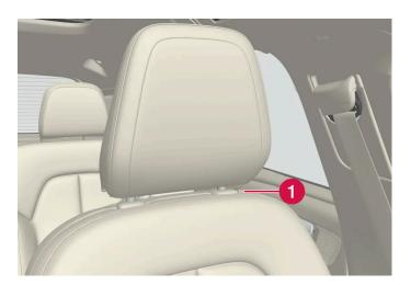
1 You can manually adjust the height of the head restraints by pressing in the button.
