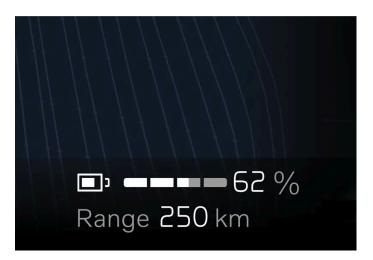
When the car is delivered from the factory, the range is based on the certified value. When the car has been driven for a while, the range is based on historical driving patterns.
