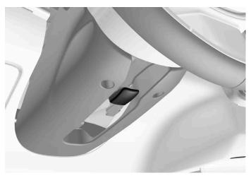
Lever for steering wheel adjustment.
