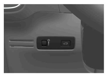
Thumbwheel (to left) for adjusting interior brightness.
