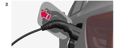
Unplug the charging cable from the car's charging input socket and close the hatch.
