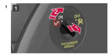
Pull the switch outward and turn from ON to OFF.
