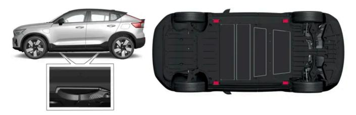
The triangles in the plastic cover indicate the locations of the lifting points (marked in red).
