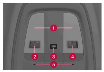
Lighting and controls in the roof console.
