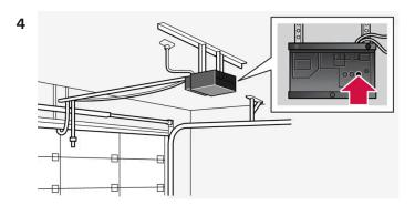
Locate programming button <sup>[2]</sup> on the receiver for the garage door or similar. It is normally located close to the antenna's bracket on the receiver.
