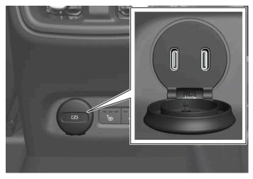
$\ensuremath{\mathsf{USB}}$  ports (type C) in the tunnel console, rear seat.
