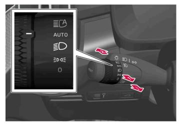
Steering wheel stalk switch with rotating ring.
