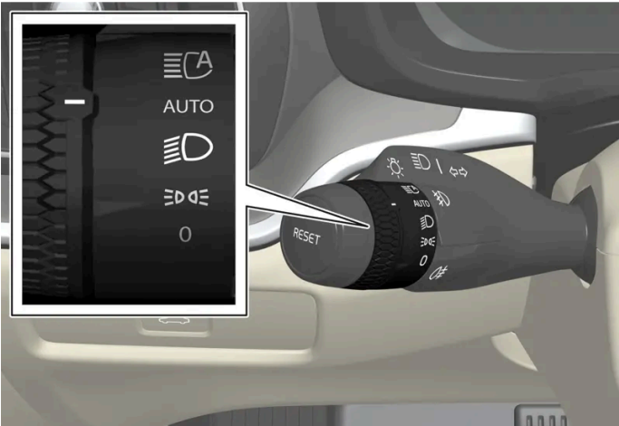
Rotating ring in the left-hand stalk switch.
