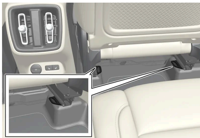
Mounting point locations in the rear seat.
