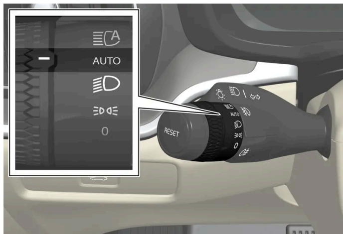
Stalk switch rotating ring in AUTO position.
