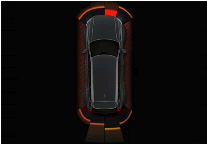
Example of screen view with obstacle zones and sensor sectors.
