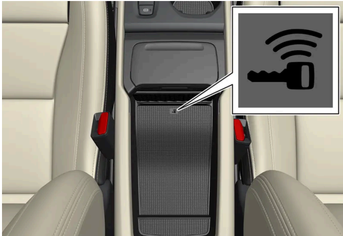
Backup reader's location in the tunnel console.
