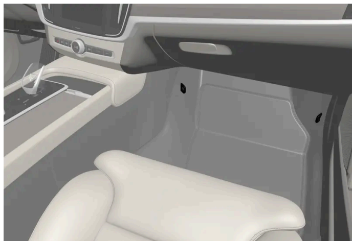
Mounting point locations in the front seat.
