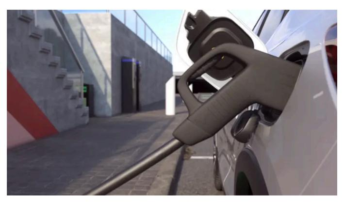
1 Detach the charging cable from the charging station's storage socket. Note that the car must be switched off prior to charging.
