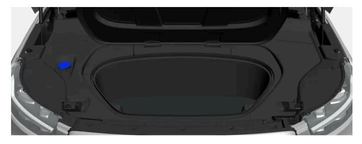
There is additional storage space under the bonnet. The car's towing eye and emergency puncture repair kit are also stored in the cargo area.
