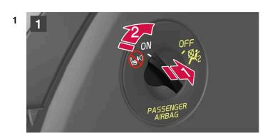
Pull the switch outward and turn from ON to OFF.
