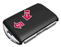
Refit the rear shell in reverse order to how it was removed. There is no logotype on the rear shell. Press in the shell until you hear a click, and then slide it the last few millimetres to its original position.
