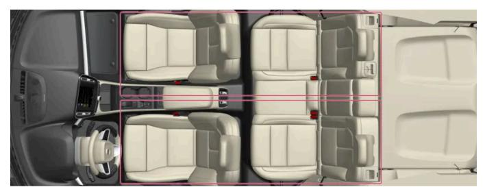
With 2-zone climate, the temperature in the passenger compartment can be set separately for the left and right-hand sides.
