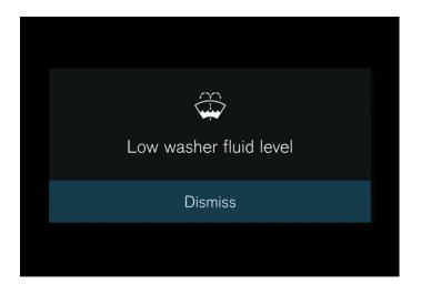
Messages are shown in the middle of the driver display. The composition may vary and is shown together with graphics, symbols or buttons for acknowledging the message or accepting a request, for example.
