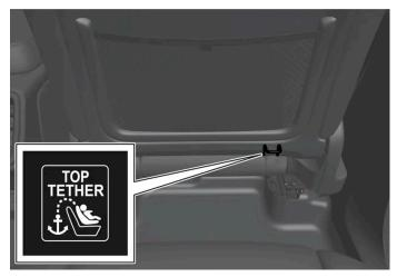
Mounting point location for the front seat is indicated by a symbol on the rear of the front seat.
