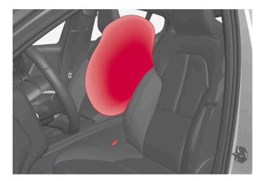
The far-side airbags are fitted in the inner backrest frames of the front seats and help to protect the driver and passengers in the front seat. The seat is marked AIRBAG.
