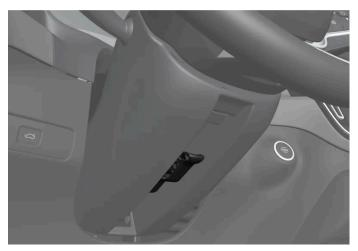
Lever for steering wheel adjustment.
