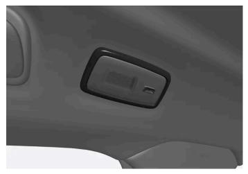
In cars with a panorama roof  $\mbox{\ensuremath{^{\star}}}$  , the two lamp units are located on either side of the roof.
