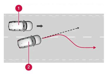
The function can assist by steering the car back to its own lane.
