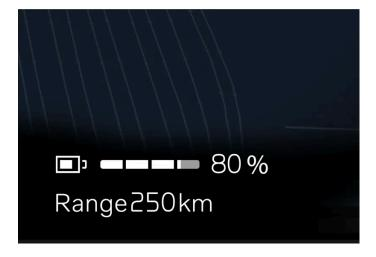
The battery gauge in the lower part of the driver display shows the State of Charge (SoC) for the high-voltage battery. This is shown next to the battery gauge when the remaining range is less than 50 km (30 miles). The range may be affected by factors such as driving style and temperature, for example.
