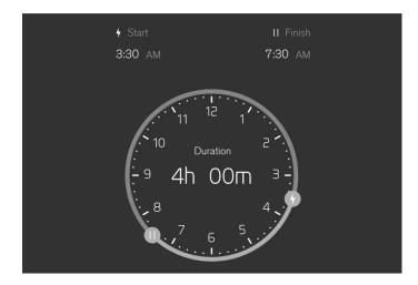
Select Charging  $\rightarrow$  Set timer in the centre display and then activate the scheduling with Schedule charging. Use the controls at  $\frac{1}{2}$  and  $\frac{1}{2}$  to set the desired start and stop time for charging.
