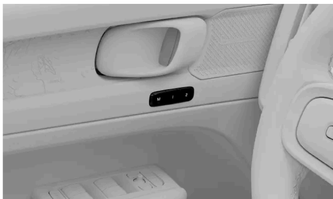
Location of the preset seat adjustment buttons
