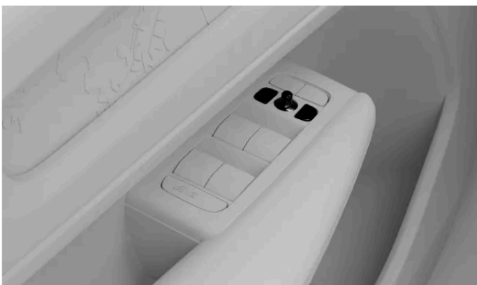
Controls for adjusting the wing mirrors
