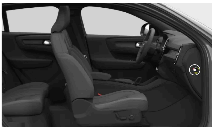
Location of the passenger airbag switch
