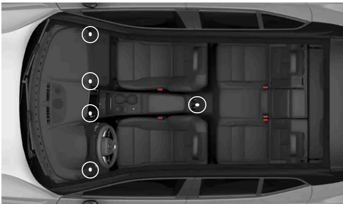
The locations of the adjustable air vents
