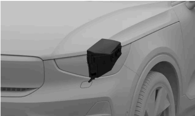
Fuse box location
