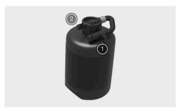
Overview of the temporary puncture repair kit's sealing fluid bottle
