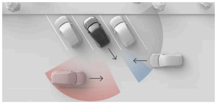
The situation shown in this image illustrates how surrounding objects, such as parked cars, can limit the radar's view. In a situation without obstacles, the effective detection zones are the same on both sides.
