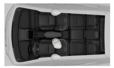
Side-on collision airbags for the front occupants.
