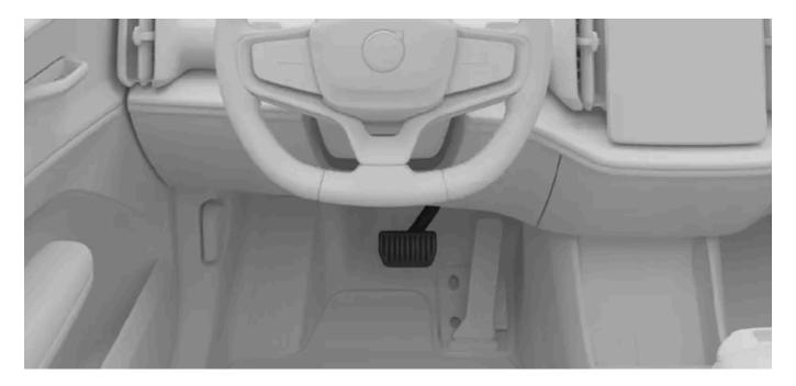
The foot brake engages either regenerative braking or the friction brakes, depending on how hard you press the pedal. Light braking activates regenerative braking, whereas harder braking engages the friction brakes.
