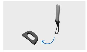
Fastening tether to lower tether anchorage point
