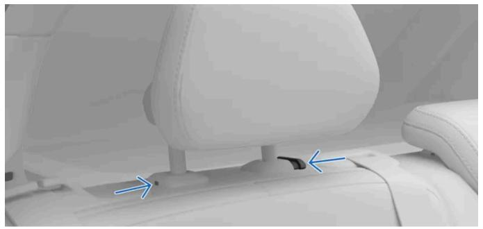
Buttons used to remove headrest.
