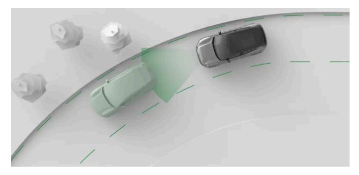
Pilot Assist actively guides your driving in a number of ways. When driving with Pilot Assist, you select the target speed. The car then manages acceleration and braking to meet that target while also adapting to surrounding traffic.
