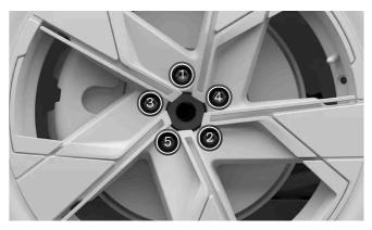
Tighten the wheel fasteners crosswise.
