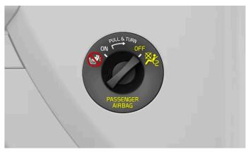
Airbag disabled. Always use this position when a rearward-facing child restraint is installed in the front passenger seat.
