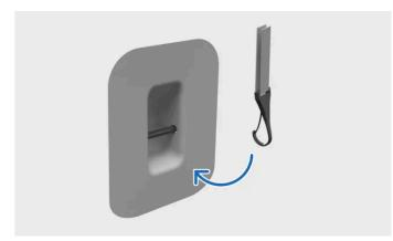
Fastening tether to top tether anchorage point
