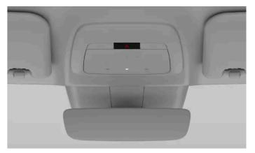
The hazard lights button is located in the overhead console. You can also access the lights in the bottom bar in the display.
