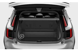
Remove the cap by prising it off with a screwdriver or a similar tool. 3
