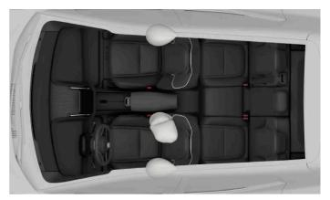
Side-on collision airbags for the front occupants.
