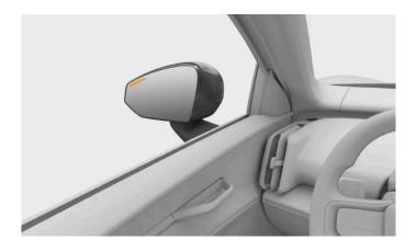
When the car detects traffic that is about to pass close to the car's sides, a light appears in the wing mirror along with a notification in the display. If you begin to open the door on the side of the detected traffic, the alert intensifies. A sound alert can occur along with the visual alerts depending on how urgent the warning is.
