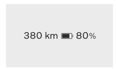
Your range is primarily related to your car's battery level and your driving practices but external conditions can also be a factor. The battery level and expected range are displayed in the driver information area. The expected range tells you how far you can drive with the current battery level. It is calculated based on your driving pattern, both current and historical, and on real-time driving conditions.
