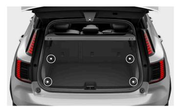
Load-retaining eyelets are located in the four corners of the boot. You can use the load-retaining eyelets to attach straps and secure cargo in the boot.
