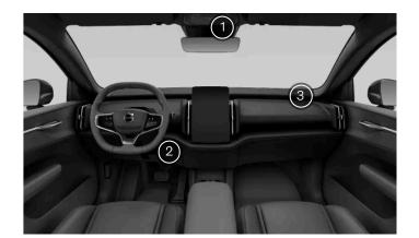
1) Sunlight, rain and humidity sensor in the rear-view mirror console.
