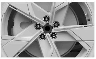
Tighten the wheel fasteners crosswise.
