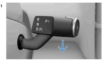
When appropriate, pull the right-hand steering wheel stalk all the way down.
