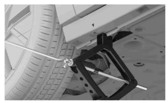
7 Raise the car to an appropriate height. Do not raise it higher than what's necessary for the work you're doing.
