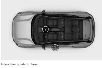
1) Key reading sensor in the driver door pillar
