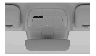
The SOS button is located in the ceiling, on the left side of the overhead console.
