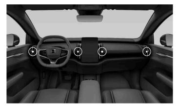
The positions of the adjustable air vents.
