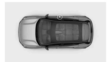
The product label is located on the right-hand door pillar and will be visible when the door is opened.
