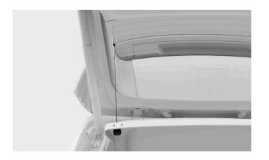
The cords have loops at each end that you hook onto the boot hatch attachment points.
