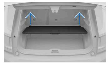
Illustrative guide for removing the cargo hatch.
