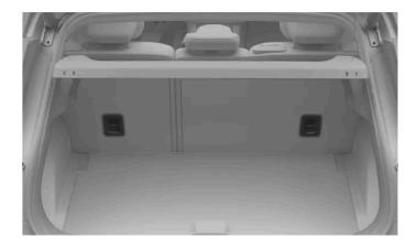
The top tether anchorage points for the rear seats are located on the back of the outer rear seats.
