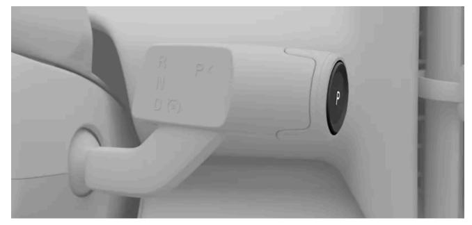
> The car transitions to a parked state, which includes engaging the parking brake. The new state is indicated in the driver information area.
