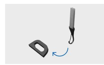
Fastening tether to lower tether anchorage point
