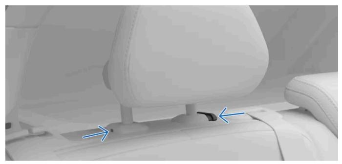
Buttons used to remove headrest.
