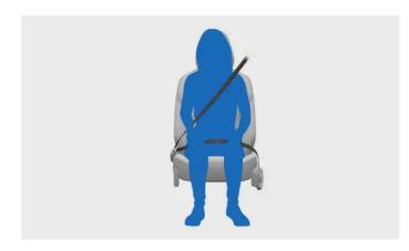
The seatbelt locks itself to act as a safety restraint under certain conditions. They include sudden and forceful pulling of the belt, if the car is driven aggressively and if the car is on a steep incline.
