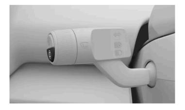
You control the rear windscreen wiper by using the lower button on the left-hand steering wheel stalk.
