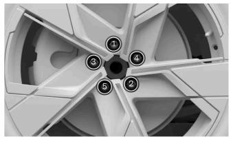
Tighten the wheel fasteners crosswise.
