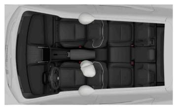
Side-on collision airbags for the front occupants.
