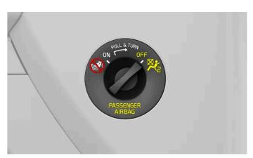
Airbag disabled. Always use this position when a rearward-facing child restraint is installed in the front passenger seat.
