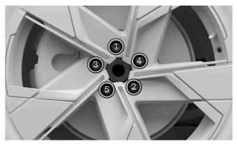
Tighten the wheel fasteners crosswise.
