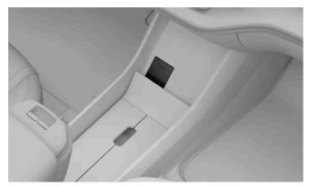
The location of the key card reader, used if you start the car with a key card or a discharged distance-capable key.
