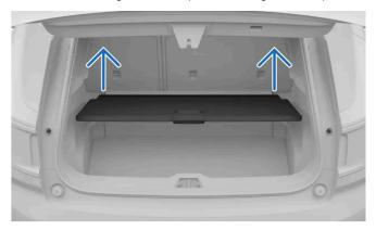
Illustrative guide for removing the cargo hatch.
