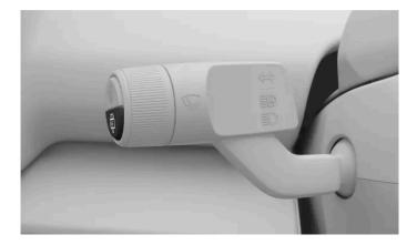
You control the rear windscreen wiper by using the lower button on the left-hand steering wheel stalk.
