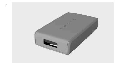
Hold the tag with the Volvo logo facing upwards. There is a small opening on one of the tag's short sides. Pry open the tag from this side by pulling the edge outwards and upwards.
