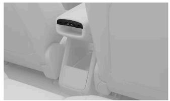
From the rear seats, you can operate the rear windows using the switches on the rear end of the centre armrest.
