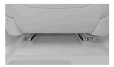
The lower tether anchorage points for the rear seats can be found at the back of the floor rails of the seats in front.
