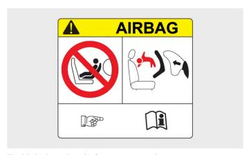
This label is located on the front passenger side sun visor.  $% \label{eq:control_passenger}$
