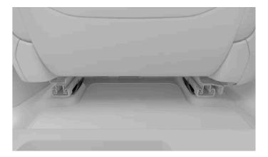
The lower tether anchorage points for the rear seats can be found at the back of the floor rails of the seats in front.
