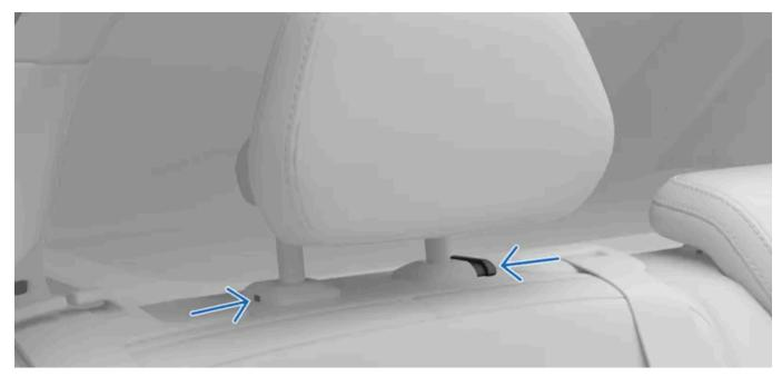
Buttons used to remove headrest.
