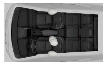
Side-on collision airbags for the front occupants.
