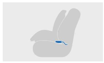
Child restraint installed using ISOFIX
