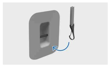
Fastening tether to top tether anchorage point
