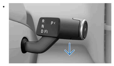
Pull the right-hand side steering wheel stalk all the way down.
