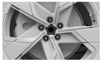
Tighten the wheel fasteners crosswise.
