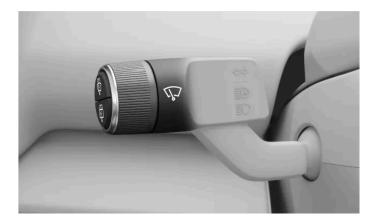
You can control the wipers and washers using the scroll wheel and buttons on the left-hand steering wheel stalk.
