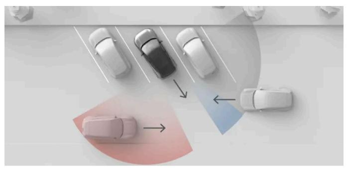
The situation shown in this image illustrates how surrounding objects, such as parked cars, can limit the radar's view. In a situation without obstacles, the effective detection zones are the same on both sides.
