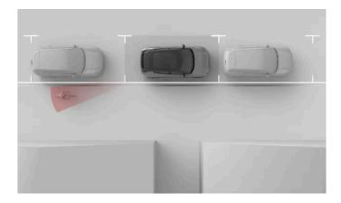
Door opening alerts are designed to warn you of passing traffic so that you don't open a door in its path. These alerts can be provided when the car is stationary or moving very slowly [1].
