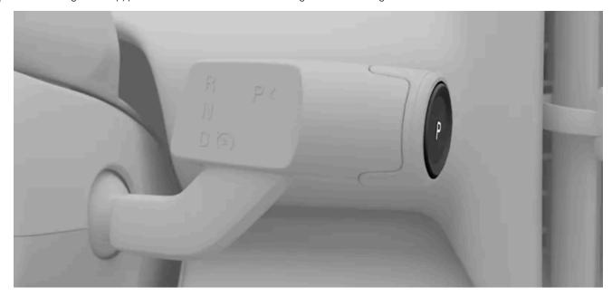
> The car transitions to a parked state, which includes engaging the parking brake. The new state is indicated in the driver information area.
