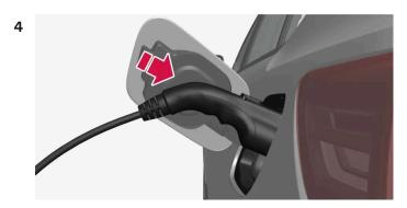
Remove the charging handle's protective cover and press the charging handle the whole way into the charging input socket.
