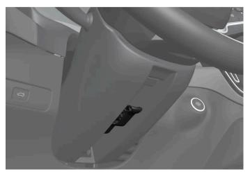
Lever for steering wheel adjustment.
