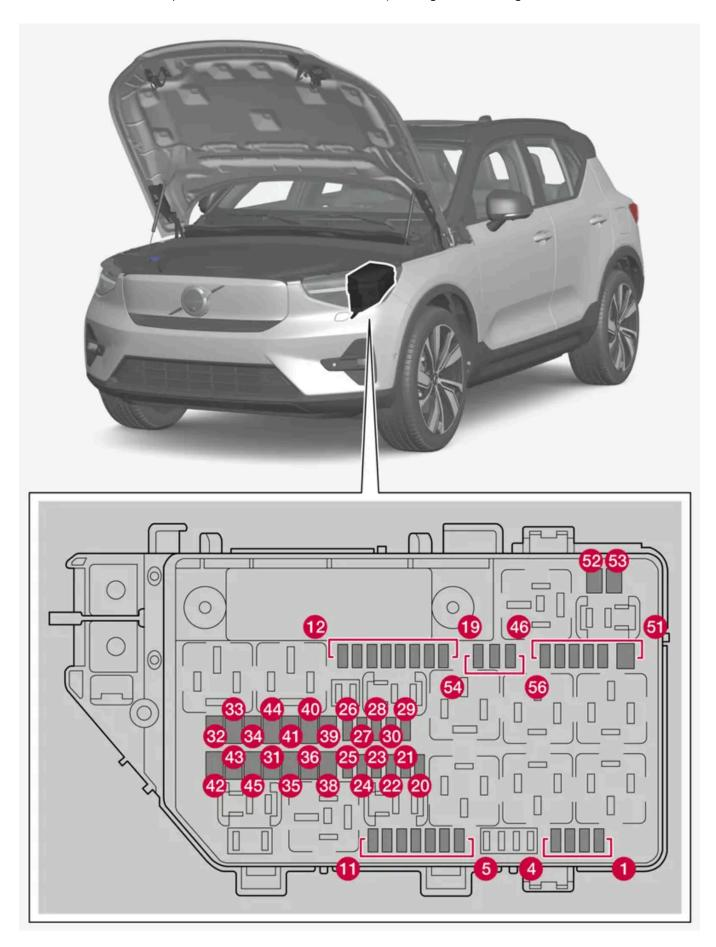
A number of panels around the storage area need to be loosened for access to fuses under the bonnet.
