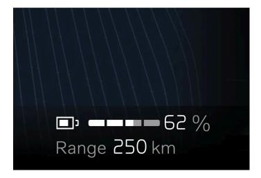
When the car is delivered from the factory, the range is based on the certified value. When the car has been driven for a while, the range is based on historical driving patterns.
