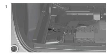
Open the car's cargo area and fold up the load floor. Lift away the recessed floor panel.
