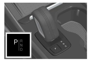
The driver display shows which gear position is currently in use.
