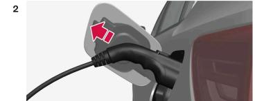
Unplug the charging cable from the car's charging input socket and close the hatch.
