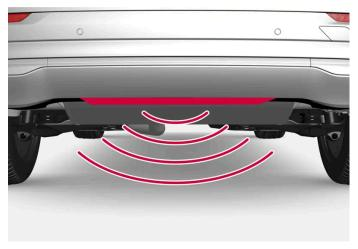
The sensor is located in the centre of the bumper.
