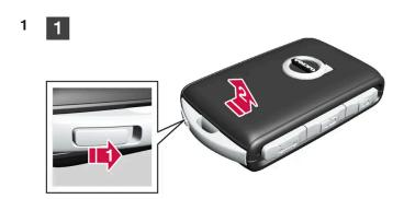
Slide the catch by the keyring bracket to the side, and slide the front shell away from the bracket.
