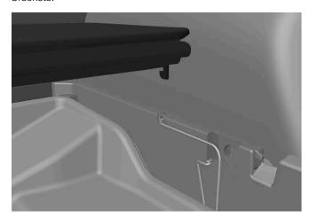
The cargo area floor can be placed carefully back onto the lock springs without being locked in position.
