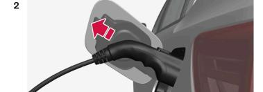
Unplug the charging cable from the car's charging input socket and close the hatch.
