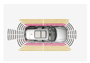
The warning signal pulses intensively at less than approx.  $25\ cm$  (0.8 foot) from an obstacle.
