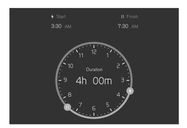
Select Charging → Set timer in the centre display and then activate the scheduling with Schedule charging. Use the controls at 4 and 11 to set the desired start and stop time for charging.
