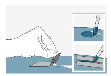
If the damage has not reached down to the metal, the touch-up paint can be applied directly after the surface has been cleaned.
