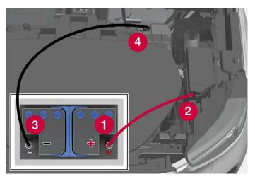
Several of the panels around the storage area need to be loosened for access to the charging points under the bonnet.
