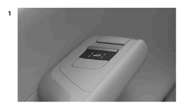
Press the window symbol at to switch between controlling the front and rear windows. The current window selection is indicated by the lights next to the symbol.
