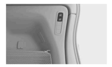
On the right-hand side in the boot, there is a button panel. The top two buttons, one for each seat, can be used to fold and raise the third row seats. This location can be useful if you need more room for stowing while using the boot.
