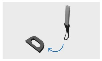
Fastening tether to lower tether anchorage point
