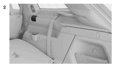
Remove the indentation covers in the sides of the rear boot.
