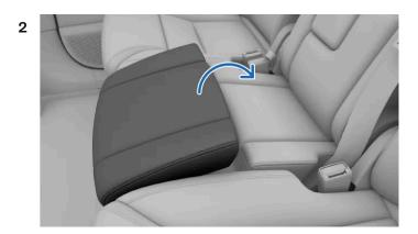
Using one hand on the front of the child seat and one on the rear, guide the child seat upwards and back all the way to the backrest of the seat.
