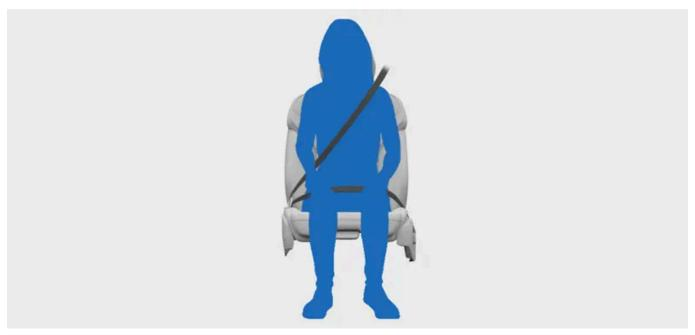
Correctly fastened and adjusted seatbelt.
