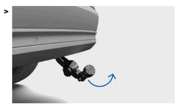
The towbar is deployed. As the towbar extends, the symbol on the deployment button flashes.
