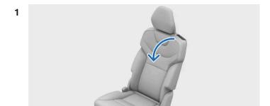
Pull the handle on the top of the outer seat backrest.
