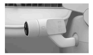
• Press and hold the button on the left-hand steering wheel stalk for the washers you want to activate. The front washers are activated by the upper button and the rear washer is activated by the lower button.
