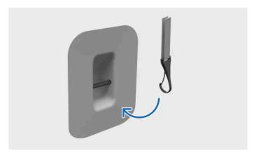
Fastening tether to top tether anchorage point
