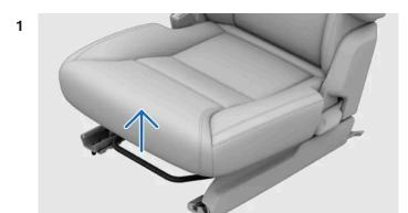
Grasp and pull the handle under the seat cushion upwards.
