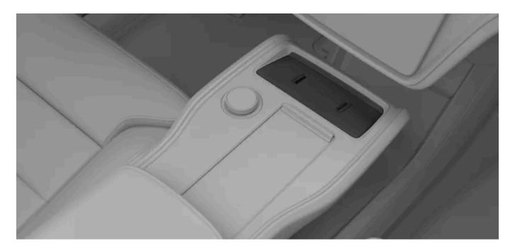
To use the wireless charger, your device should be certified to the Qi wireless charging standard. Also make sure that wireless charging is enabled on both the device [1] and on the charger itself. You can enable the charger in the centre display.
