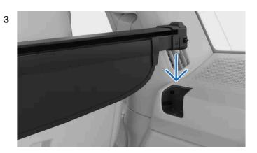
Push the load cover into the indentations until both sides of the load cover click into place. Ensure the locks are positioned so that the red marks are covered.
