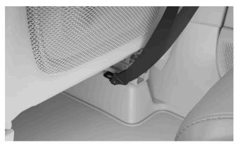
Tighten the straps to make the safety net tight and more secure.
