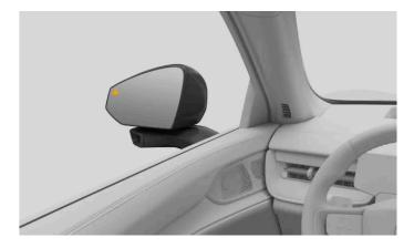
When the car detects traffic that is about to pass close to the car's sides, a light appears in the wing mirror. If you begin to open the door on the side of the detected traffic, the alert intensifies. A sound alert can occur along with the visual alerts depending on how urgent the warning is.
