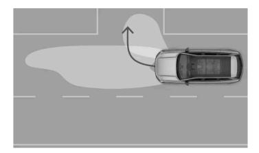
The cornering lights illuminate the area close to the car to give you better visibility when turning.
