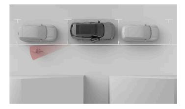
Door opening alerts are designed to warn you of passing traffic so that you don't open a door in its path. These alerts can be provided when the car is stationary or moving very slowly [1].
