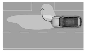
The static bending lights trigger when turning
