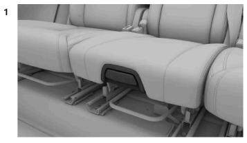
Pull the handle on the front of the centre seat cushion to release the lock.
