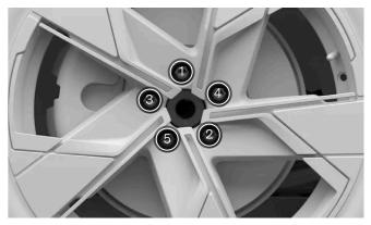
Tighten the wheel fasteners crosswise.
