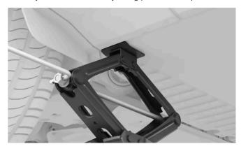
8 Raise the car to an appropriate height. Do not raise it higher than what's necessary for the work you're doing.
