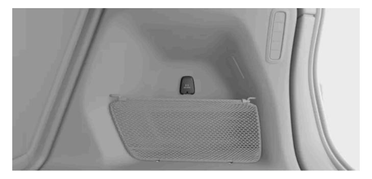
The 12 V electrical socket is on the right-hand side in the boot.
