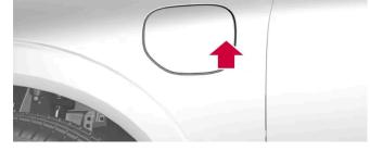
Press in the rear section of the cover to open the charging hatch<sup>[2]</sup>.
