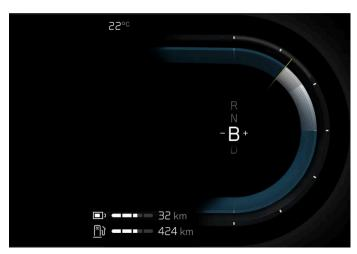
Gear shift indicator in the driver display.
