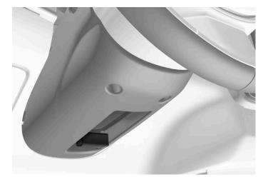
Lever for steering wheel adjustment.
