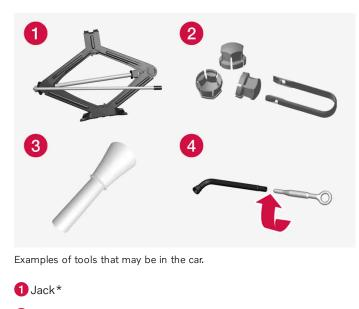
**2** Tool for removing the plastic caps from the wheel bolts
