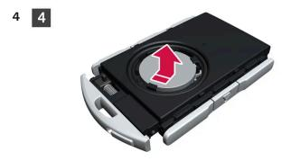
The battery (+) side is facing upwards. Loosen the battery by pressing on its edge and then lifting it out.
