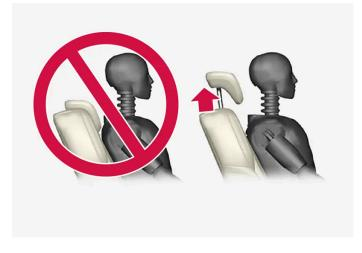
The centre seat's head restraint must be adjusted according to the passenger's height so that, if possible, the whole of the back of the head is covered. Slide it up manually as required.
