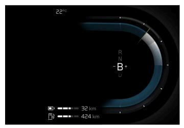
Gear shift indicator in the driver display.
