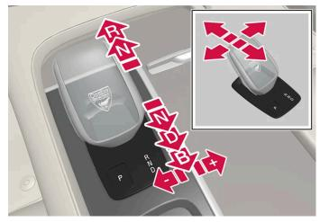
Overview of gear lever and gear positions.
