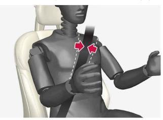
The seatbelt must pass over the shoulder (not down over the arm).
