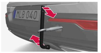
Screw the eye in firmly. For example, thread through the wheel bolt wrench\* and use it as a lever.
