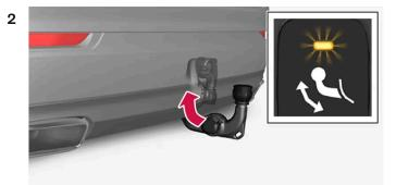
Lock the towbar by moving it back to its retracted position, where it is locked.
