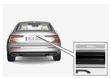
Rubberised pressure plate on the boot lid can only be used for unlocking.
