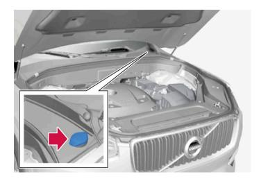
Washer fluid is filled into the reservoir with the blue cap. The reservoir is used for both windscreen washer and headlamp washers\*.
