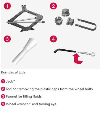
If the car is fitted with a spare wheel\*, there is a jack and a wheel bolt wrench instead of emergency puncture repair kit.
