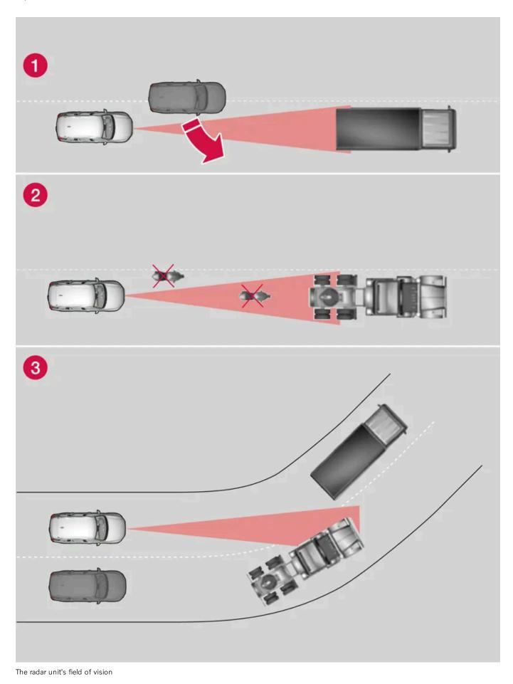
Sometimes the radar unit is late at detecting vehicles at close distances - e.g. a vehicle that drives in between your car and the vehicle ahead.
