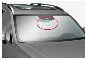
Location of front camera and radar unit
