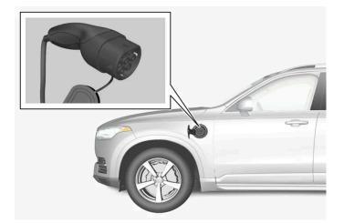
Charging cable handle and charging input socket.
