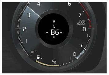
Gear shift indicator in the driver display<sup>[1]</sup>.
