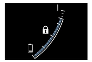
The f symbol in the hybrid battery gauge indicates that the Hold function is activated, and the **f** symbol indicates that the **Charge** function is activated.
