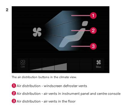
Press one or more of the air distribution buttons in order to open/close the corresponding air flow.
