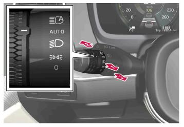
Steering wheel stalk switch with rotating ring.
