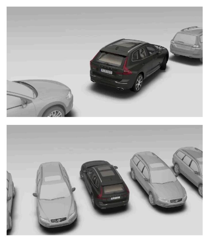
The function first checks if a space is large enough and if so then assists the driver to steer the car into the space.
