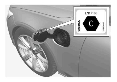
Use charging that is approved for use in the car in accordance with the identifier<sup>[1]</sup> on the inside of the charging input socket flap.
