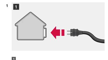
Connect the charging cable to a 230 V socket. Never use an extension cable.
