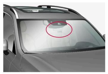
Location of front camera and radar unit
