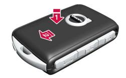
Refit the front shell in reverse order to how it was removed. Press in the shell until you hear a click, and then slide it the last few millimetres to its original position.
