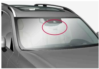
Location of front camera and radar unit
