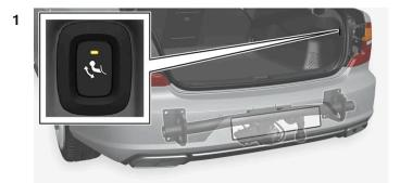
Open the boot lid. A button for extending/retracting the towbar is located on the right-hand side at the rear of the cargo area. An indicator lamp in the button must illuminate with a constant orange glow for the extension function to be active.
