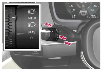
Steering wheel stalk switch with rotating ring.
