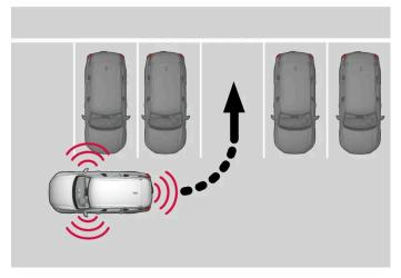
Principle for reversing into perpendicular parking.
