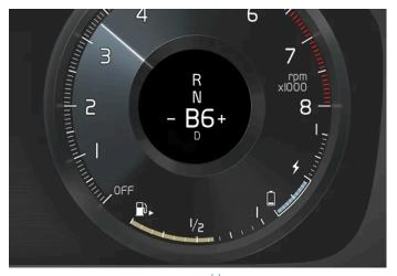
Gear shift indicator in the driver display<sup>[1]</sup>.
