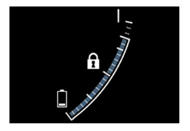
The f symbol in the hybrid battery gauge indicates that the Hold function is activated, and the f symbol indicates that the Charge function is activated.
