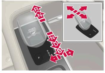
Overview of gear lever and gear positions.
