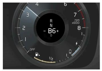
Gear shift indicator in the driver display<sup>[1]</sup>.
