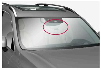
Location of front camera and radar unit
