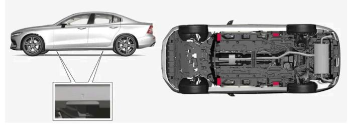
Arrows along the bottom edge of the side of the car mark where the jacking points/lifting points (marked in red) are located.
