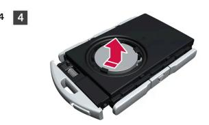
The battery (+) side is facing upwards. Loosen the battery by pressing on its edge and then lifting it out.
