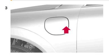
Press in the rear section of the cover to open the charging hatch<sup>[2]</sup>.
