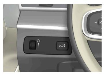
Thumbwheel (to left) for adjusting interior brightness.
