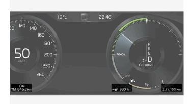
Examples of trip computer information in the driver display. The figure is schematic - parts may vary depending on car model.
