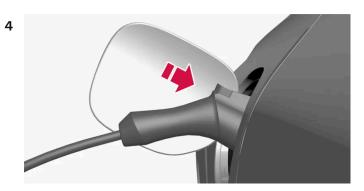
Remove the charging handle's protective cover and press the charging handle the whole way into the socket for the car.
