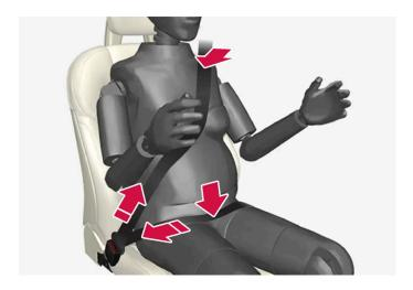
The diagonal section should wrap over the shoulder then be routed between the breasts and to the side of the abdomen.
