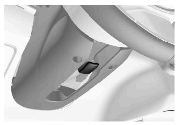
Lever for steering wheel adjustment.
