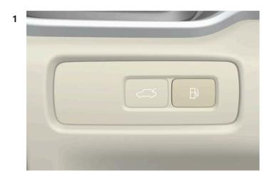
Press the button on the instrument panel.
