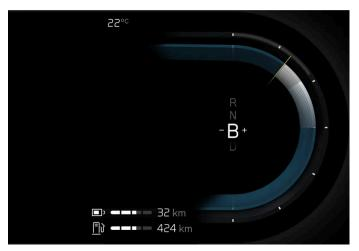
Gear shift indicator in the driver display.
