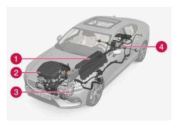
1 Hybrid battery - The function of the hybrid battery is to store energy. It receives energy when charging from the mains power circuit, during regenerative braking or from the high-voltage generator. It provides energy for electric operation as well as for temporarily operating the electric air conditioning during the preconditioning of the passenger compartment.
