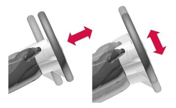
The steering wheel can be adjusted for height and for depth.
