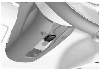
Lever for steering wheel adjustment.
