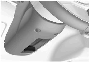
Lever for steering wheel adjustment.
