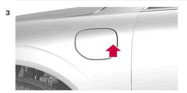
Press in the rear section of the cover to open the charging hatch [2].
