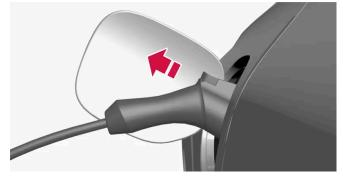
Unplug the charging cable from the car's charging input socket and close the hatch.
