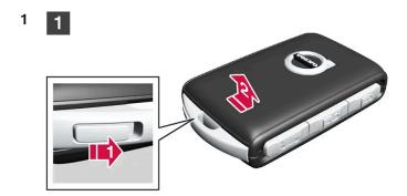
Slide the catch by the keyring bracket to the side, and slide the front shell away from the bracket.
