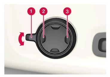
$\label{eq:Multi-function} \mbox{ Multi-function button, located on the side of the seat base section.}$
