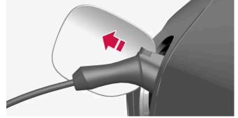
Unplug the charging cable from the car's charging input socket and close the hatch.
