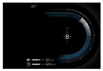
Gear shift indicator in the driver display.
