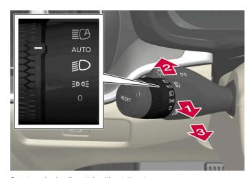
Steering wheel stalk switch with rotating ring.
