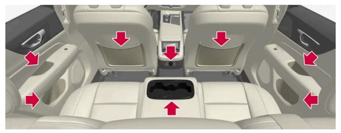
Storage compartment in the door panel, cup holder\* in the centre seat backrest, storage pocket\* on the front seat backrest, as well as USB ports in the tunnel console.
