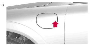
Press in the rear section of the cover to open the charging hatch<sup>[2]</sup>.
