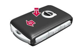
Refit the front shell in reverse order to how it was removed. Press in the shell until you hear a click, and then slide it the last few millimetres to its original position.
