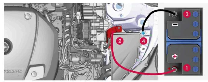
Charging points for jump starting own car. The appearance in the engine compartment may vary depending on car model and equipment level.
