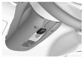
Lever for steering wheel adjustment.
