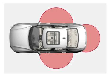
For keyless use, a key must be within a distance of approx. 1 to 1.5 metres (3 to 5 feet) from the car's doors or boot lid.
