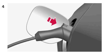
Remove the charging handle's protective cover and press the charging handle the whole way into the socket for the car.
