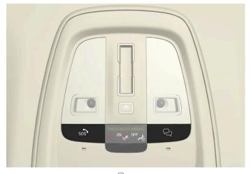
The functions are available via the  $\ensuremath{\mathbb{Q}}$  and SOS buttons in the car's roof.
