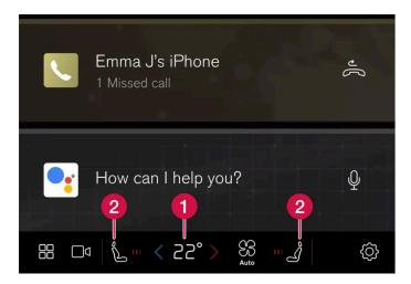
**1** Temperature controls for driver and passenger side.<sup>[1]</sup>
