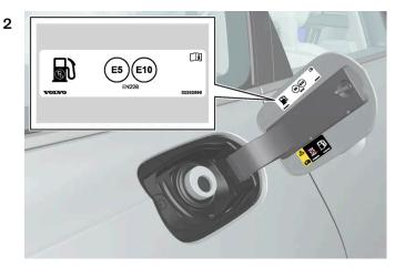
Choose fuel that is approved for use in the car in accordance with the identifier<sup>[1]</sup> on the inside of the fuel filler flap. See information on approved fuels and identifier in the section on "Petrol".
