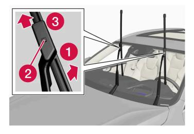
Make sure that the windscreen wipers are in service position and fold up the wiper arms. Service position is activated/deactivated via the centre display when the car is stationary and the windscreen wipers are not switched on.
