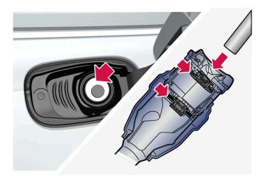
It is important to feed the pump nozzle past the filler pipe's two openable hatches before starting to fuel the car.
