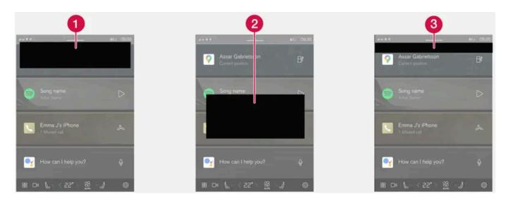
• Appears at the top of the centre display. Requires direct action and can have up to three buttons that allow the user to deal with the message. Dismiss by sweeping right or left, the message is then saved in notification view.
