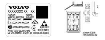
CEM marking for the remote control key system. For supplementary type approval numbers, see following tables.
