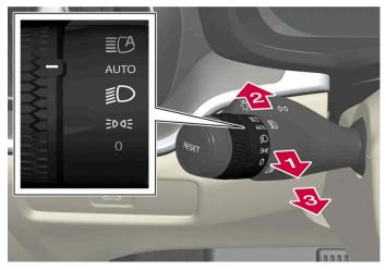
Steering wheel stalk switch with rotating ring.
