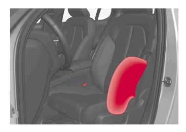
The near-side airbags are fitted in the outer backrest frames of the front seats and help to protect the driver and passengers in the front seat.
