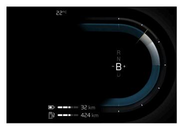
Gear shift indicator in the driver display.
