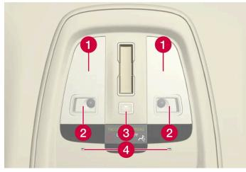
Lighting and controls in the roof console.
