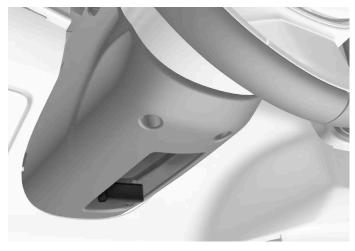
Lever for steering wheel adjustment.
