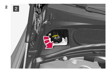
Screw off the cap and top up with coolant if necessary. The coolant level must lie between the  $\mbox{MIN}$  and  $\mbox{MAX}$  marks on the expansion tank.
