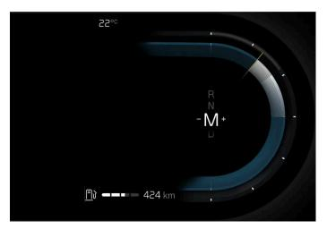
Gear shift indicator in the driver display.
