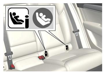
Mounting point locations for the rear seat are indicated by symbols [1] on the covers that conceal the mounting points.
