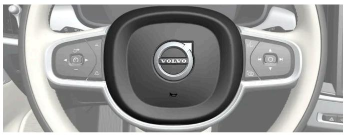
The horn is located in the centre of the steering wheel.
