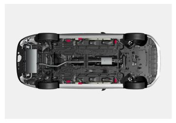
The car has outer lifting points for low level lifting, and inner lifting points for high level lifting, such as garage jack or lifting arms.
