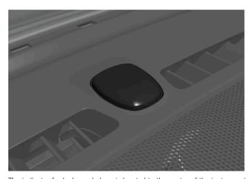
$\label{the control of the instrument panel, close to the windscreen.} The indicator for locks and alarm is located in the centre of the instrument panel, close to the windscreen.}$
