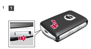
Slide the catch by the keyring bracket to the side, and slide the front shell away from the bracket.
