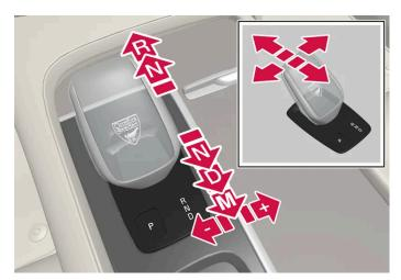
Overview of gear lever and gear positions.
