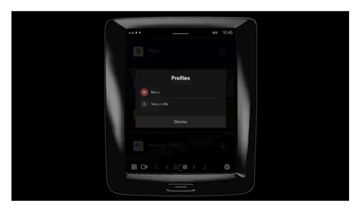
The Owner profile is pre-installed and active in the car on first use or after a factory reset.
