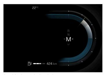
Gear shift indicator in the driver display.
