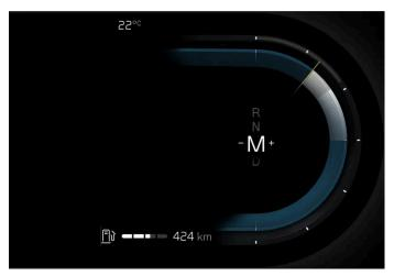
Gear shift indicator in the driver display.
