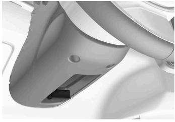
Lever for steering wheel adjustment.
