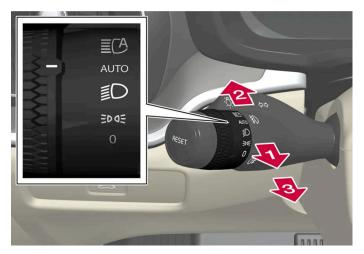
Steering wheel stalk switch with rotating ring.
