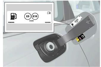
Choose fuel that is approved for use in the car in accordance with the identifier [1] on the inside of the fuel filler flap. See information on approved fuels and the identifier in the section on "Petrol".
