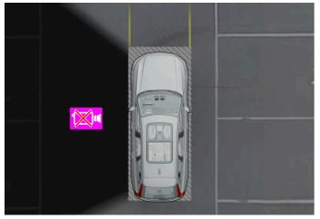
Example for showing when the car's left camera is non-operational.
