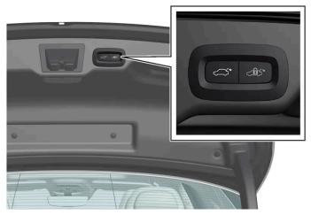
Location of button on the underside of the boot lid.
