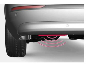
The sensor is positioned to the left of centre in the bumper.
