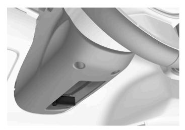
Lever for steering wheel adjustment.
