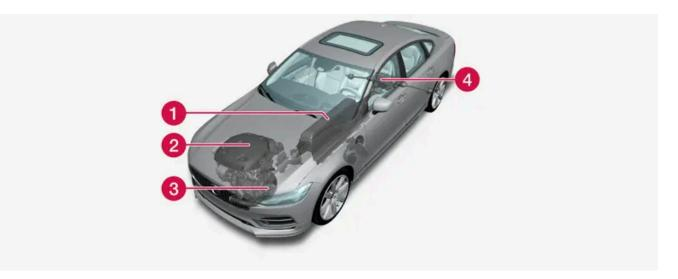
Hybrid battery - The function of the hybrid battery is to store energy. It receives energy when charging from the mains power circuit, during regenerative braking or from the high-voltage generator. It provides energy for electric operation as well as for temporarily operating the electric air conditioning during the preconditioning of the passenger compartment.
