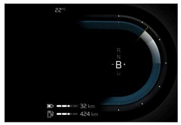
Gear shift indicator in the driver display.
