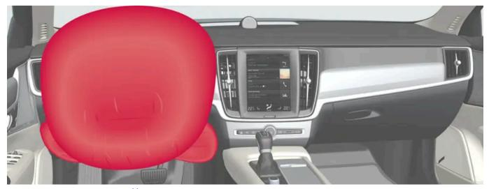
Steering wheel airbag and knee airbag<sup>[1]</sup> on the driver's side in the front seat.
