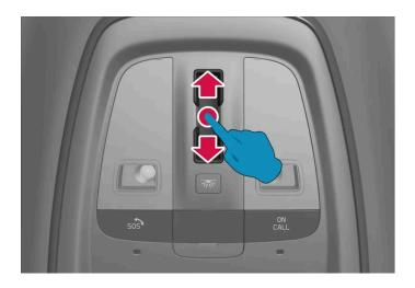
Open the sunroof – swipe backwards over the control. The sunroof first reaches comfort position<sup>[1]</sup>. In order to open to maximum opening position – swipe over the control backwards a second time.
