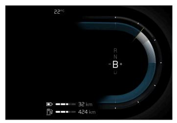
Gear shift indicator in the driver display.
