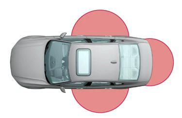
For keyless use, a key must be within a distance of approx. 1 to 1.5 metres (3 to 5 feet) from the car's doors or boot lid.
