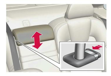
To lower the head restraint, the button (see illustration) must be depressed while the restraint is carefully moved down.
