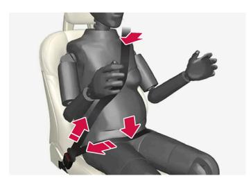
The diagonal section should wrap over the shoulder then be routed between the breasts and to the side of the abdomen.
