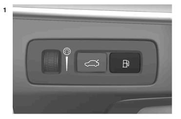
Press the button on the instrument panel.
