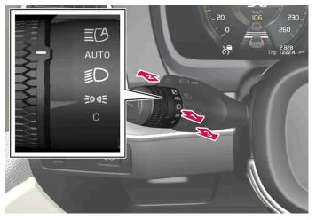
Steering wheel stalk switch with rotating ring.
