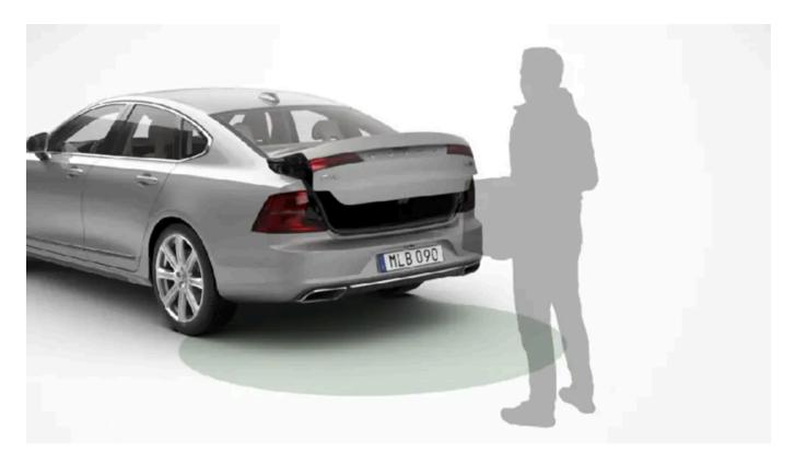
If the car is equipped with keyless locking and unlocking\* then you can open the boot lid with a foot movement. For closing, the car also needs to be equipped with power operated boot lid\*.
