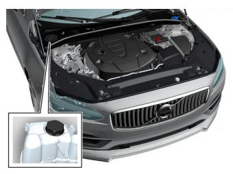
Coolant expansion tank, left-hand drive car.
