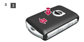
Refit the front shell in reverse order to how it was removed. Press in the shell until you hear a click, and then slide it the last few millimetres to its original position.
