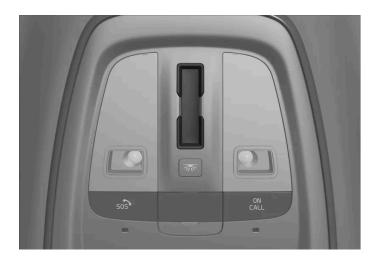
The sunroof is operated with a control located in the roof. The control is activated when the car's electrical system is in ignition position | or ||.
