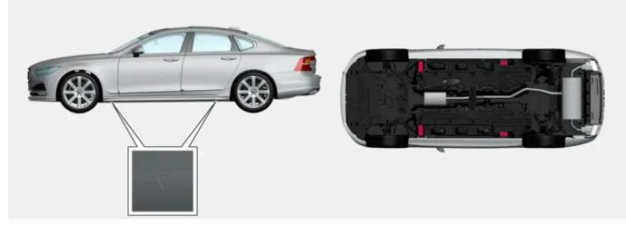
The triangles in the plastic cover indicate the locations of the lifting points (marked in red).
