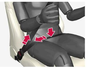
The hip strap must be positioned low down (not over the abdomen).
