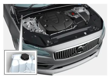
Coolant expansion tank, right-hand drive car
