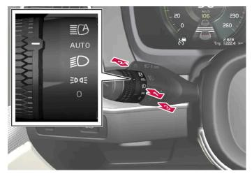
Steering wheel stalk switch with rotating ring.
