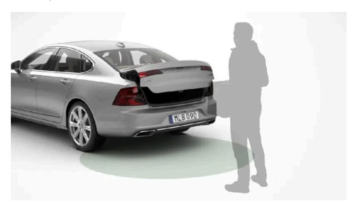
If the car is equipped with keyless locking and unlocking\* then you can open the boot lid with a foot movement.
