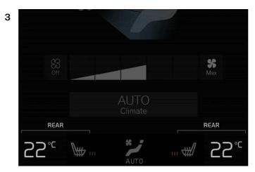
Temperature buttons in the Rear climate tab in the climate view.
