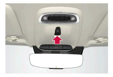
The sunroof is operated with a control located in the roof. The control is activated when the car's electrical system is in ignition position | or ||.
