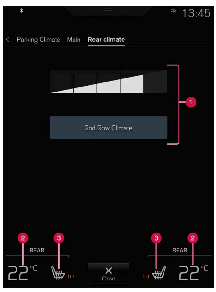
12nd row climate - Controls for climate functionality in the rear seat. Fan controls for rear seat.
