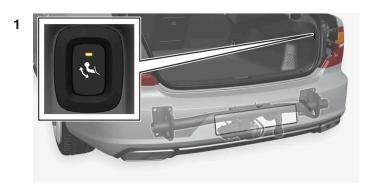
Open the boot lid. A button for extending/retracting the towbar is located on the right-hand side at the rear of the cargo area. An indicator lamp in the button must illuminate with a constant orange glow for the extension function to be active.
