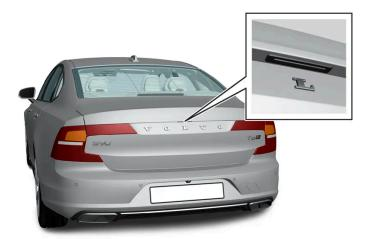
Rubberised pressure plate on the boot lid can only be used for unlocking.
