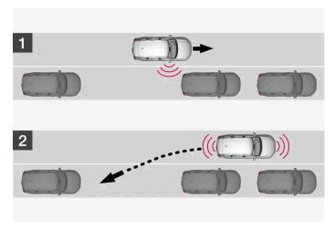
Principle for reversing into parallel parking.
