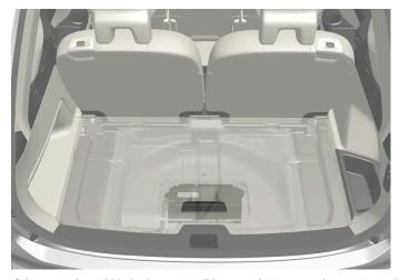
If the car is the mild hybrid type, it will have a 48 V support battery instead, located under the cargo area. The box over the 48 V support battery must only be handled by an authorised workshop.
