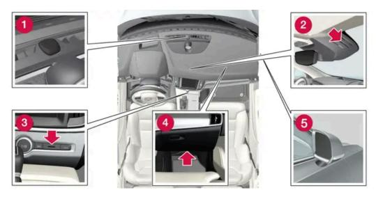
1 Sun sensor - on the upper side of the instrument panel.
