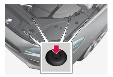
Press down the pins into the plastic cover's four clips using a screwdriver or similar and lift away the cover.
