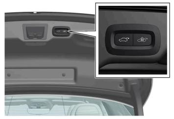
Location of button on the underside of the boot lid.
