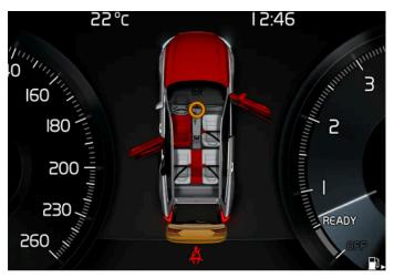
Graphics in the driver display with different types of warnings. The warning colour on the door and boot lid is dependent on the speed of the car.
