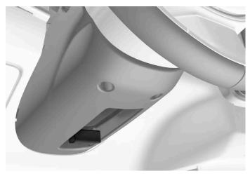
Lever for steering wheel adjustment.
