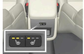
Buttons for heated seats at the rear of the tunnel console.
