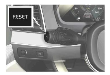
1 Reset all information in trip meter TM (i.e. mileage, average consumption, average speed and driving time) with a long press on the RESET button on the left-hand stalk switch.
