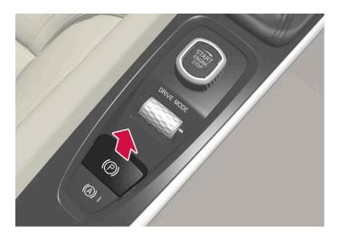
1 Pull the control upward.
