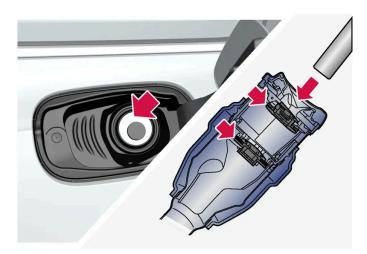
It is important to feed the pump nozzle past the filler pipe's two openable hatches before starting to fuel the car.  $\frac{1}{2} \int_{\mathbb{R}^{n}} \frac{1}{2} \int_{\mathbb{R}$
