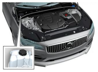
Coolant expansion tank, left-hand drive car
