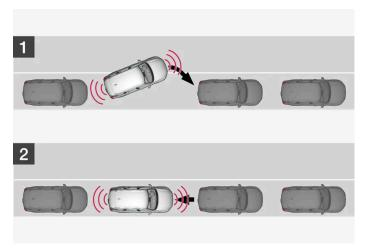
Principle for positioning during parallel parking.
