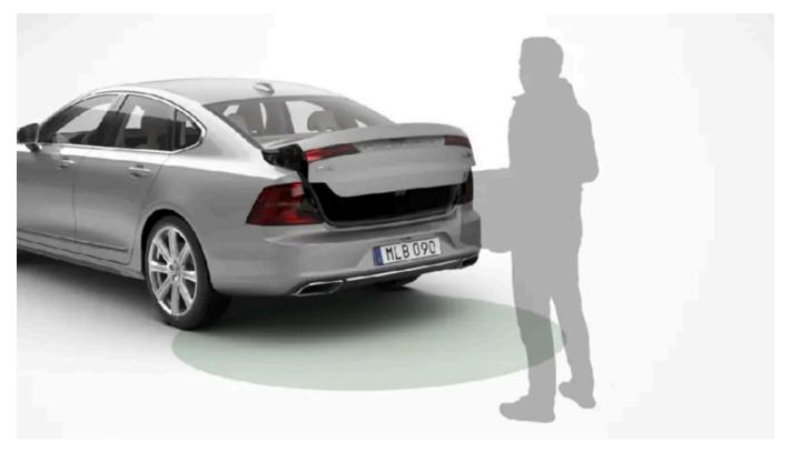
If the car is equipped with keyless locking and unlocking\* then you can open the boot lid with a foot movement.
