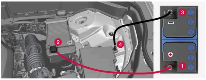
Attachment points for the jump leads. The appearance in the engine compartment may vary depending on car model and equipment level.
