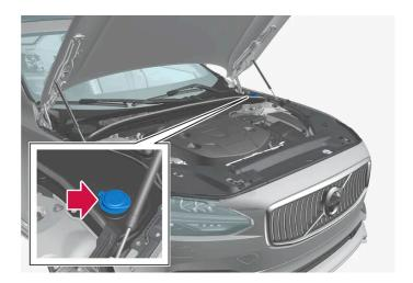
Washer fluid is filled into the reservoir with the blue cap. The reservoir is used for both windscreen washer and headlamp washers\*.
