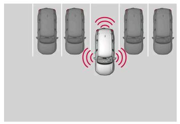
Principle for positioning during perpendicular parking.
