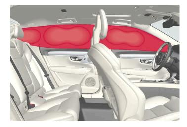
The inflatable curtain is mounted along both sides of the headlining and helps protect the driver and outer seat passengers of the car. The panels are labelled with IC AIRBAG.
