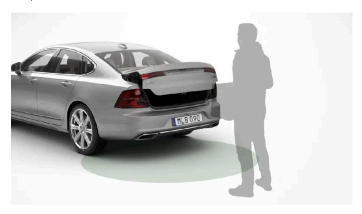
If the car is equipped with keyless locking and unlocking\* then you can open the boot lid using a foot movement. For closing, the car also needs to be equipped with power operated boot lid\*.
