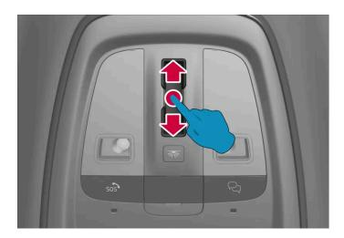
Open the sunroof – swipe backwards over the control. The sunroof first reaches comfort position [1]. In order to open to maximum opening position – swipe over the control backwards a second time.
