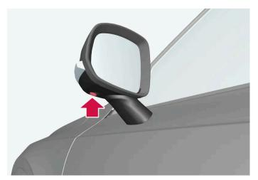
The side cameras are positioned in each door mirror.
