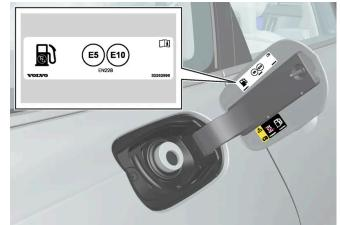
Choose fuel that is approved for use in the car in accordance with the identifier [1] on the inside of the fuel filler flap. See information on approved fuels and the identifier in the sections on "Petrol" and "Diesel" respectively.
