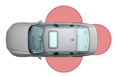
For keyless use, a key must be within a distance of approx. 1 to 1.5 metres (3 to 5 feet) from the car's doors or boot lid.
