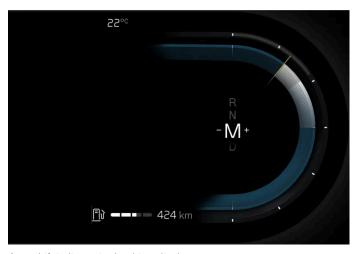
Gear shift indicator in the driver display.
