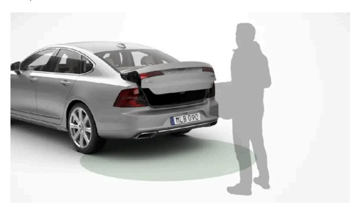
If the car is equipped with keyless locking and unlocking\* then you can open the boot lid using a foot movement. For closing, the car also needs to be equipped with power operated boot lid\*.
