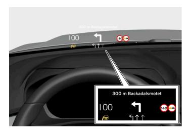
The head-up display projects information from the driver display onto the windscreen in front of the driver. The information can only be seen from the driver's position.
