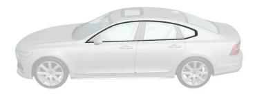
Parts that should be washed using a cleaning agent with a pH value between 3.5 and 11.5.
