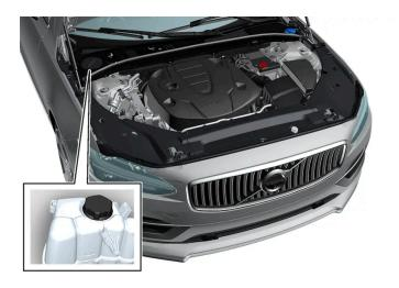
Coolant expansion tank, left-hand drive car.
