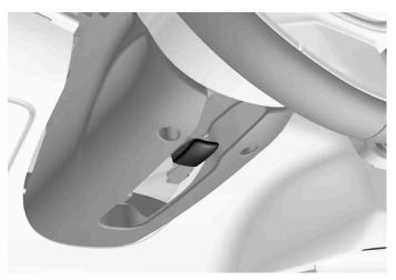
Lever for steering wheel adjustment.
