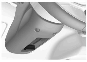
Lever for steering wheel adjustment.
