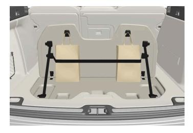
There are two bag hooks and an elastic strap [1] in the cover, which is part of the floor hatch in the cargo area. The strap can be fitted in four different positions.
