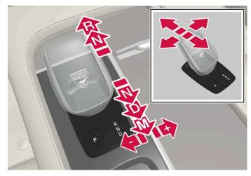
Overview of gear lever and gear positions.
