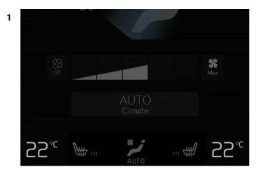
Press the left or right-hand side temperature button in the centre display's climate row to open the controls.
