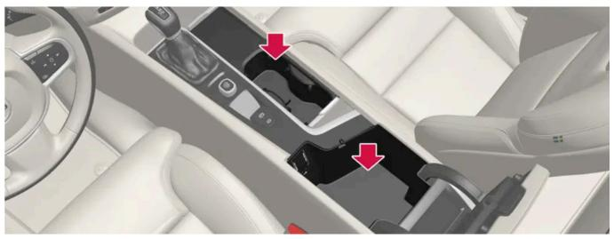
Storage spaces with cup holder, electrical socket, wireless phone charger\*, as well as USB ports in the tunnel console.
