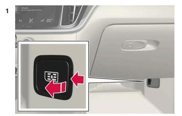
Fit a personal SIM card into the holder by the floor on the passenger side.
