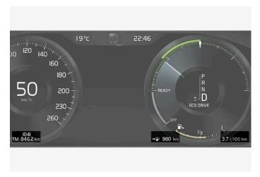
Examples of trip computer information in the 12-inch driver display\*. The figure is schematic - parts may vary depending on car model.
