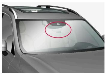
Location of front camera and radar unit
