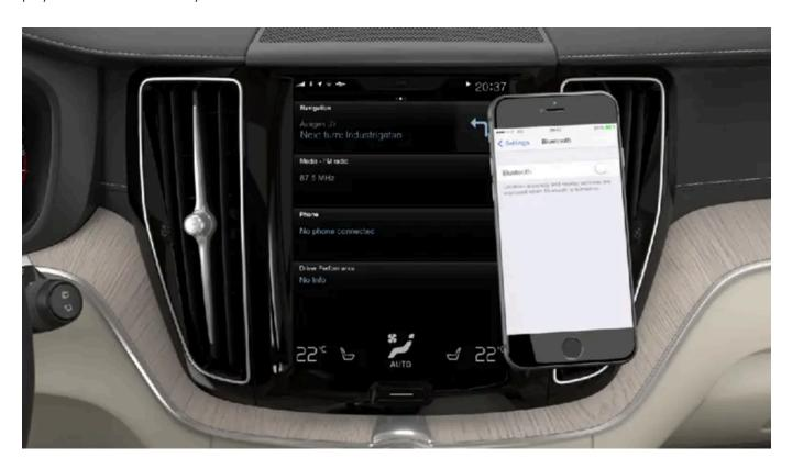
It is possible to have two Bluetooth devices connected at once, in which case one of them can only play back wirelessly. The most recently connected phone will automatically be connected to make calls, send/receive messages, play back media and provide an Internet connection [1]. It is possible to change what the phone is to be used for under **Bluetooth Devices** via the settings menu in the centre display's top view. Your mobile phone needs to be equipped with Bluetooth and support tethering.
