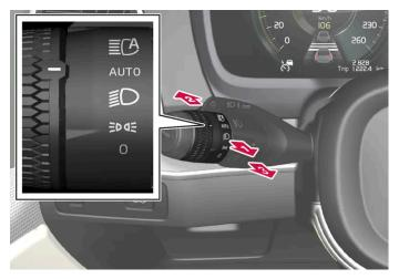
Steering wheel stalk switch with rotating ring.
