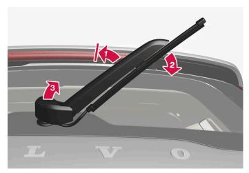
Lift the wiper arm from the windscreen and pull the upper section of the blade diagonally down to the right.
