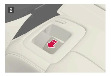
For cars without electronic folding, the outer head restraints are folded manually using the inner control on the upper side of the seat; see figure 2.
