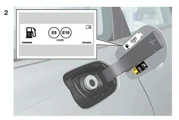
Choose fuel that is approved for use in the car in accordance with the identifier on the inside of the fuel filler flap. See information on approved fuels and the identifier in the sections on "Petrol" and "Diesel" respectively.
