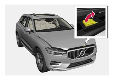
2 Sweep from left to right in the opening under the bonnet, move the handle up and to the side to release catch and lift the bonnet.
