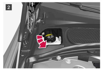
Screw off the cap and top up with coolant if necessary. The coolant level must lie between the MIN and MAX marks on the expansion tank.
