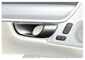
Opening handle for alternative unlocking in the side door<sup>[1]</sup>.
