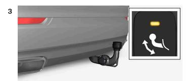
Move the towbar to its end position, where it is secured and locked in place - the indicator lamp illuminates with a constant orange glow.
