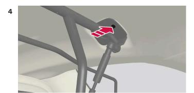
Insert the supplied screw and tighten using the supplied 6 mm Allen key. Repeat on the other side. Recommended tightening torque: 20 Nm (15 foot-pounds).
