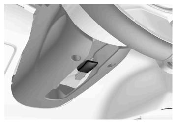
Lever for steering wheel adjustment.
