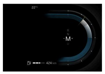
Gear shift indicator in the driver display.
