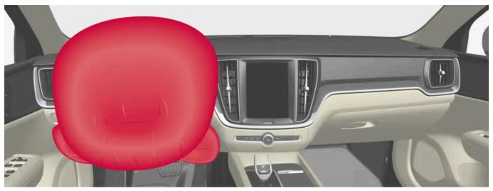
Steering wheel airbag and knee airbag  $\ensuremath{^{[1]}}$  on the driver's side in the front seat.
