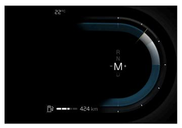
Gear shift indicator in the driver display.
