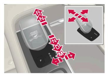
Overview of gear lever and gear positions.
