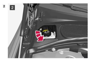
Screw off the cap and top up with coolant if necessary. The coolant level must lie between the MIN and MAX marks on the expansion tank.
