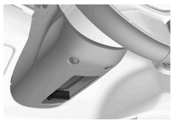
Lever for steering wheel adjustment.
