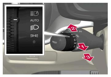
Steering wheel stalk switch with rotating ring.
