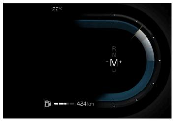
Gear shift indicator in the driver display.
