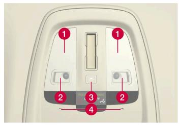
Lighting and controls in the roof console.
