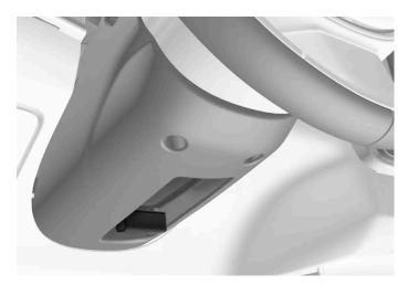
Lever for steering wheel adjustment.
