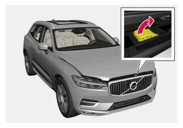
😢 Sweep from left to right in the opening under the bonnet, move the handle up and to the side to release catch and lift the bonnet.
