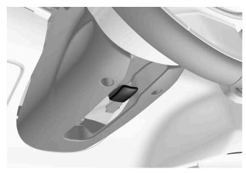
Lever for steering wheel adjustment.
