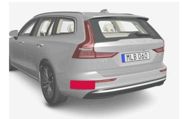
Keep the surface indicated clean - on both the left and right-hand sides of the car
