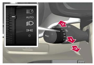
Steering wheel stalk switch with rotating ring.
