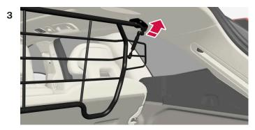
Position the safety grille's brackets on the roof mountings.
