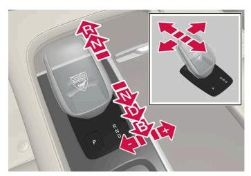
Overview of gear lever and gear positions.
