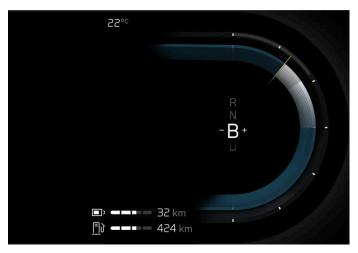
Gear shift indicator in the driver display.
