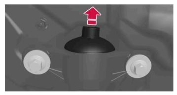
The rubber cover is located above the adjuster knob.
