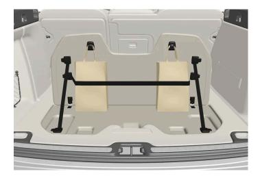
There are two bag hooks and an elastic strap [1] in the cover, which is part of the floor hatch in the cargo area. The strap can be fitted in four different positions.
