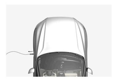
The hybrid battery is charged via a charging cable, but can be charged by gentle braking and engine braking in gear position B. The hybrid battery can also be charged by the car's engine. The car's starter battery is charged when the hybrid battery is charging.
