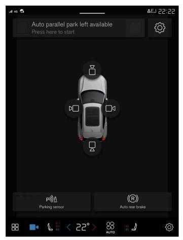
Camera view shows the park assist cameras (PAC $^{[1]}$ ), which displays a composite 360° view and separate views for each of the four cameras: rear, front, left or right camera view.
