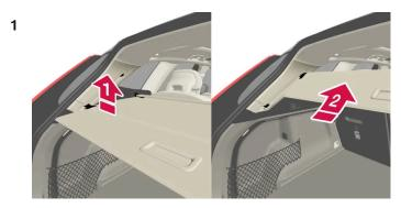
Press the cargo cover's handle section upwards slightly.
