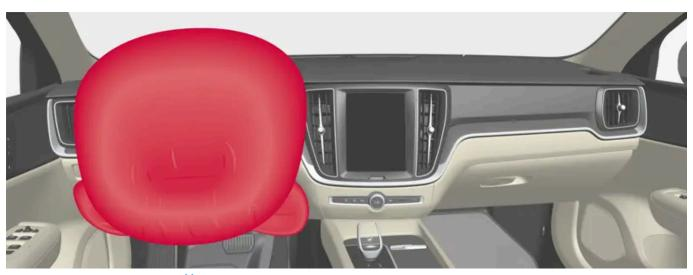
Steering wheel airbag and knee airbag [1] on the driver's side in the front seat.
