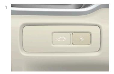
Press the button on the instrument panel.
