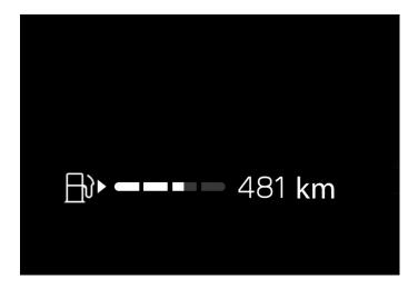
The white zone in the fuel gauge indicates the quantity of fuel in the tank.
