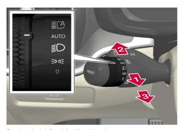
Steering wheel stalk switch with rotating ring.
