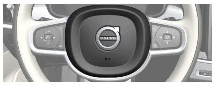
The horn is located in the centre of the steering wheel.
