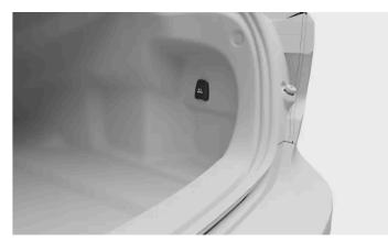
The 12 V electrical socket on the right-hand side in the boot
