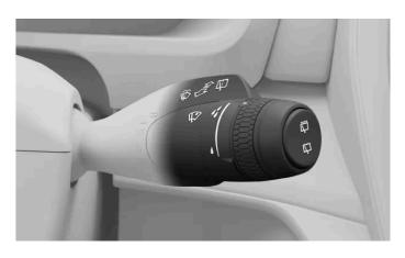
You control the wipers and washers using the right-hand steering wheel stalk.
