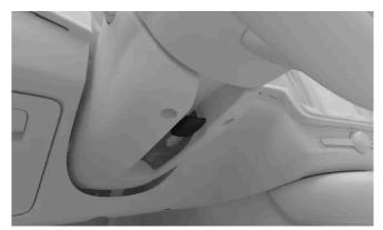
**2** Grasp the steering wheel and adjust its position.
