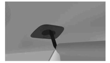
6 Fasten the lower corners of the net to the load-retaining eyelets behind the seats.
