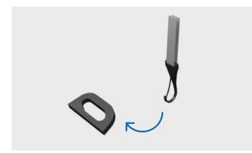
Fastening tether to lower tether anchorage point
