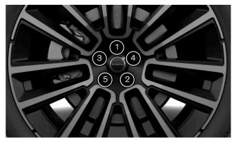
Tighten the wheel fasteners crosswise.
