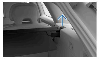
Lift the load cover completely from the indentations at the back of the boot to remove it.
