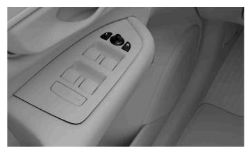
Controls for adjusting the wing mirrors
