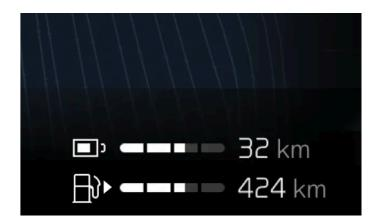
Your range is primarily related to your car's battery, the amount of fuel left in your car's tank and your driving practices but external conditions can also be a factor. The battery level and expected range are displayed in the driver display. The expected range is calculated based on your driving pattern, both current and historical.
