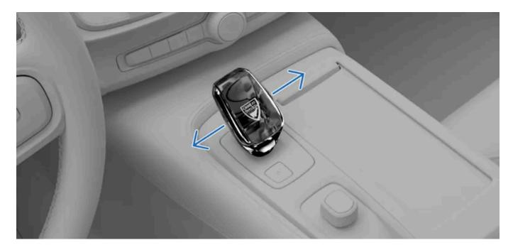
After selecting gear B, you can manually shift gears by moving the gear selector to the left or right.
