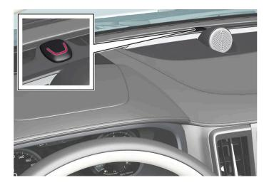
A red LED on the instrument panel indicates the alarm system's status:
