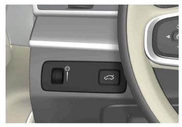
Thumbwheel (to left) for adjusting interior brightness.
