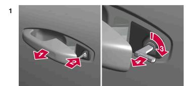
Pull out the front door handle on the left-hand side to its end position so that the lock cylinder becomes visible [1].
