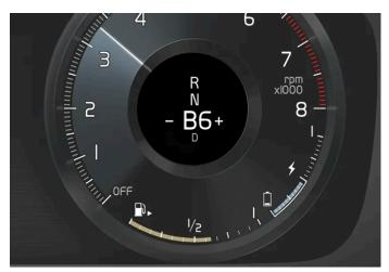
Gear shift indicator in the driver display [1].
