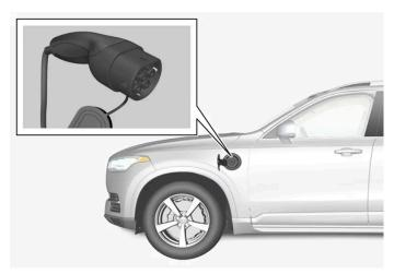
Charging cable handle and charging input socket.
