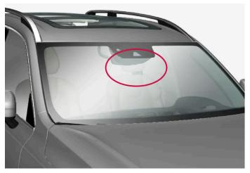
Location of front camera and radar unit
