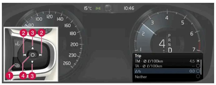
Open and navigate in the app menu  $\ensuremath{^{[1]}}$  using the right-hand steering wheel keypad.
