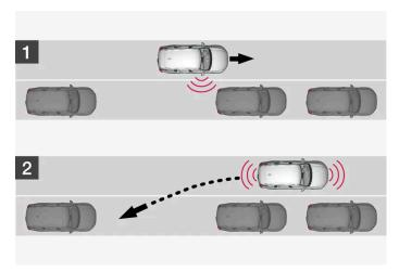
Principle for reversing into parallel parking.
