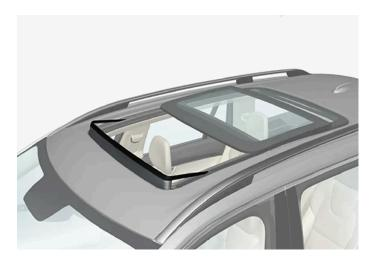
The panoramic roof has a wind deflector that is raised when the panoramic roof is in the open position.
