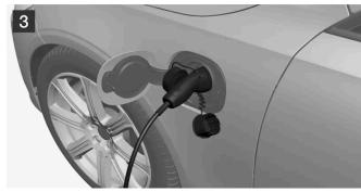
Position the charging handle's protective cover so that it does not touch the car.
