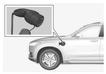
Charging cable handle and charging input socket.
