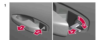
Pull out the front door handle on the left-hand side to its end position so that the lock cylinder becomes visible [1].
