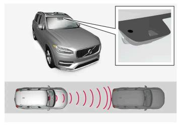
The camera and radar unit measures the distance to the vehicle ahead.
