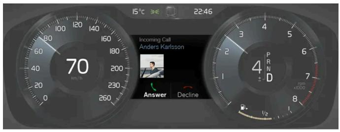
Examples of messages in the driver display. The figure is schematic - parts may vary depending on car model.
