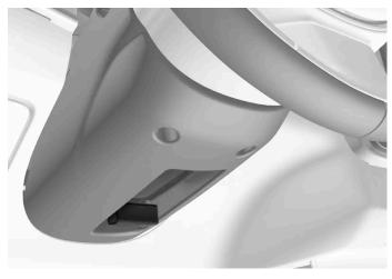
Lever for steering wheel adjustment.
