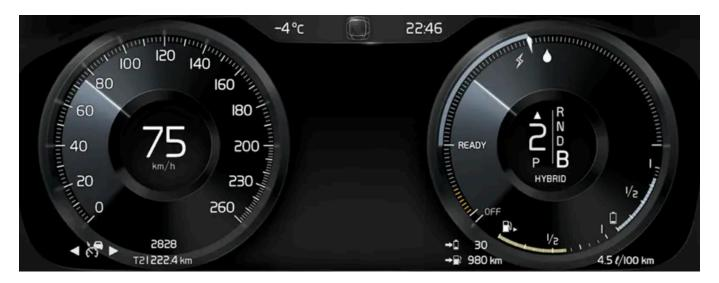
The driver display shows information on speed and e.g. incoming calls or song tracks being played. The display is operated via the two steering wheel keypads.
