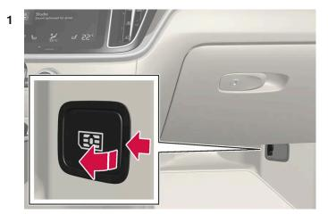
Fit a personal SIM card into the holder by the floor on the passenger side.
