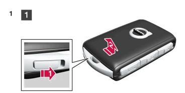
Hold the key with the front visible and the Volvo logo facing the right way - slide the button by the key ring bracket to the right. Guide the front side's shell a few millimetres upwards.
