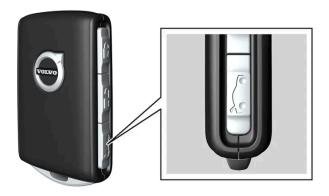
Unlocking the tailgate by pressing a button:
