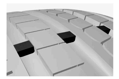
A tread wear indicator is a narrow elevation across the longitudinal grooves of the tyre's tread pattern. On the side of the tyre are the letters TWI (Tread Wear Indicator). When the tyre's tread depth is down to 1.6 mm (1/16 inch), the tread will be level in height with the tread wear indicators. Change to new tyres as soon as possible. Remember that tyres with little tread depth provide very poor grip in rain and snow.
