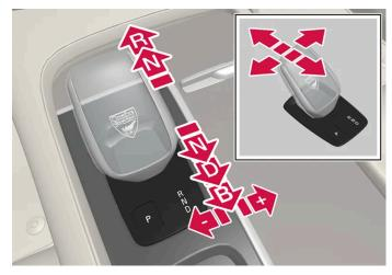
Overview of gear lever and gear positions.
