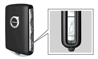
Unlocking the tailgate by pressing a button:
