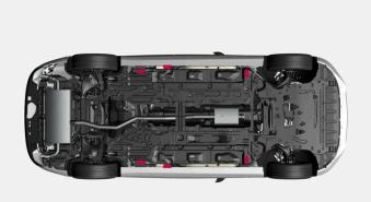
The car has outer lifting points for low level lifting, and inner lifting points for high level lifting, such as garage jack or lifting arms.
