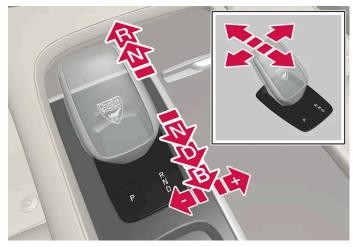
Overview of gear lever and gear positions.
