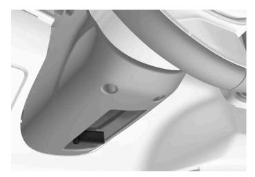
Lever for steering wheel adjustment.
