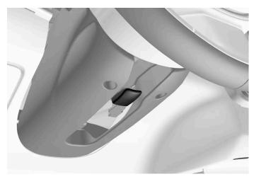
Lever for steering wheel adjustment.
