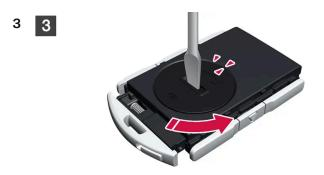
Turn the battery cover anticlockwise to OPEN position. Use a screwdriver or a coin, for example.
