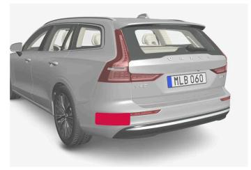
Keep the surface indicated clean - on both the left and right-hand sides of the car
