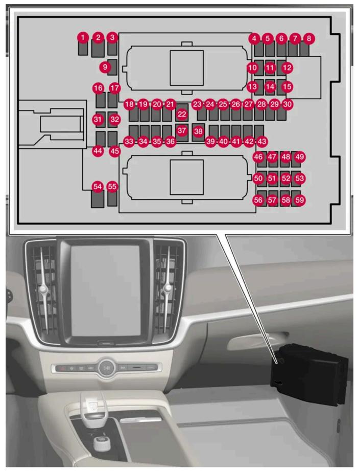
The central electrical unit is located behind the floor mat/side panel.
