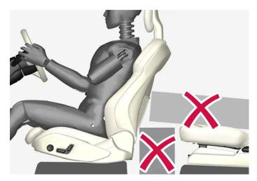
Do not leave any objects on the floor behind or under the front seats or in the rear seat that may prevent WHIPS from functioning.
