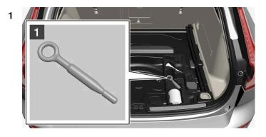
Take out the towing eye from the foam block under the floor in the cargo area.
