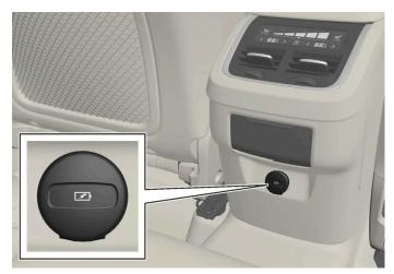
USB ports (type C) on rear of tunnel console for charging phones and tablets [1], for example.
