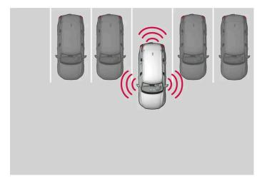
Principle for positioning during perpendicular parking.
