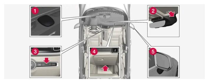
① Sun sensor - on the upper side of the instrument panel.
