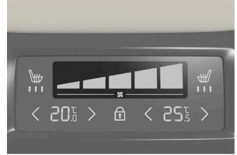
Fan controls on the climate panel at the rear of the tunnel console.
