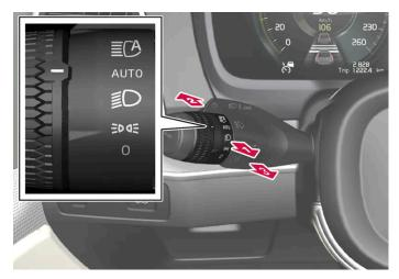
Steering wheel stalk switch with rotating ring.
