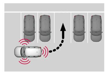
Principle for reversing into perpendicular parking.
