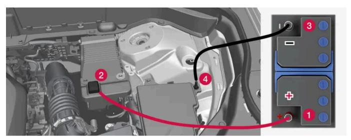
Attachment points for the jump leads. The appearance in the engine compartment may vary depending on car model and equipment level.
