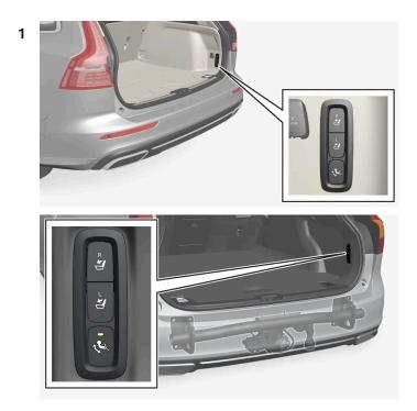
Open the tailgate. A button for extending/retracting the towbar is located on the right-hand side at the rear of the cargo area. An indicator lamp in the button must illuminate with a constant orange glow for the extension function to be active. 2 Press and release the button – extension might not start if the button is pressed for too long.
