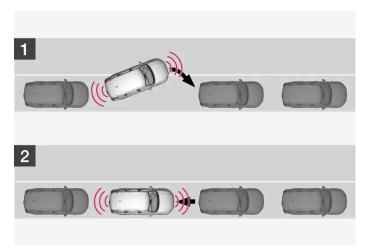
Principle for positioning during parallel parking.
