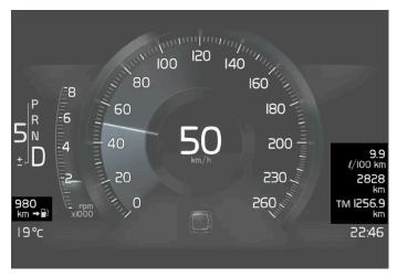
Examples of trip computer information in the 8-inch driver display. The figure is schematic - parts may vary depending on car model.
