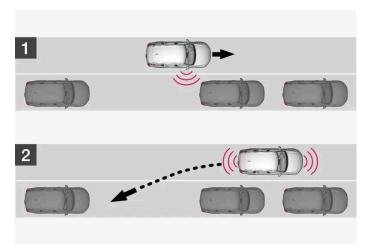
Principle for reversing into parallel parking.
