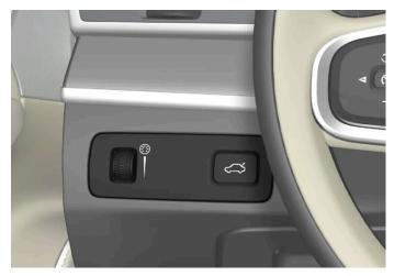
Thumbwheel (to left) for adjusting interior brightness.
