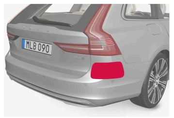
Keep the surface indicated clean – on both the left and right-hand sides of the car<sup>[2]</sup>.
