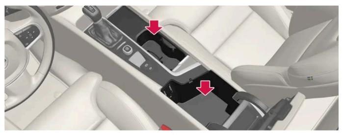
$Storage\ spaces\ with\ cup\ holder,\ electrical\ socket,\ wireless\ phone\ charger^{\star},\ as\ well\ as\ USB\ ports\ in\ the\ tunnel\ console.$
