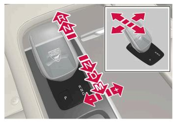
Overview of gear lever and gear positions.
