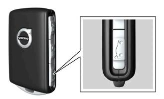
Unlocking the tailgate by pressing a button:
